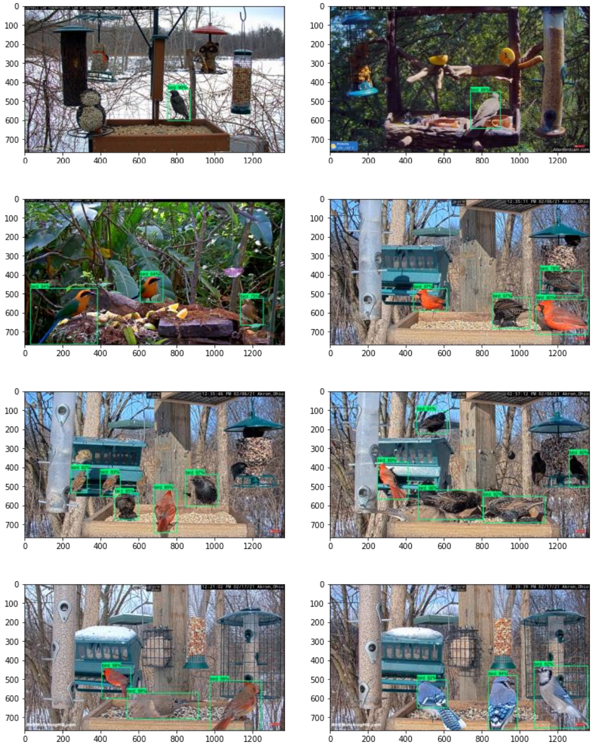
Figure 6.2: Examples of correctly detected birds by the SSD ResNet152 model.
