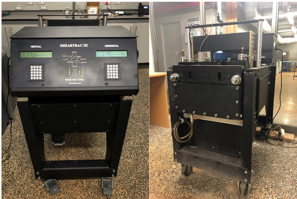
Figure 3-7 Automated large direct ShearTrac-III apparatus (Front & back).
