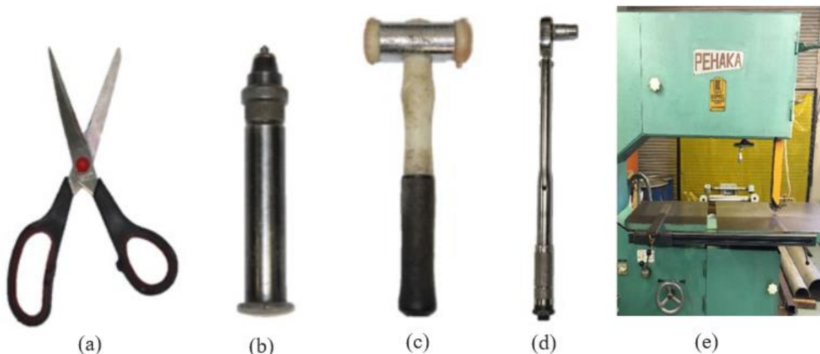
Figure 3-10 Tools and equipment used in sample preparation: (a) pair of scissors, (b) mechanical hole puncher, (c) rubber hammer, (d) ratchet bolt driver and (e) mechanical saw machine.
