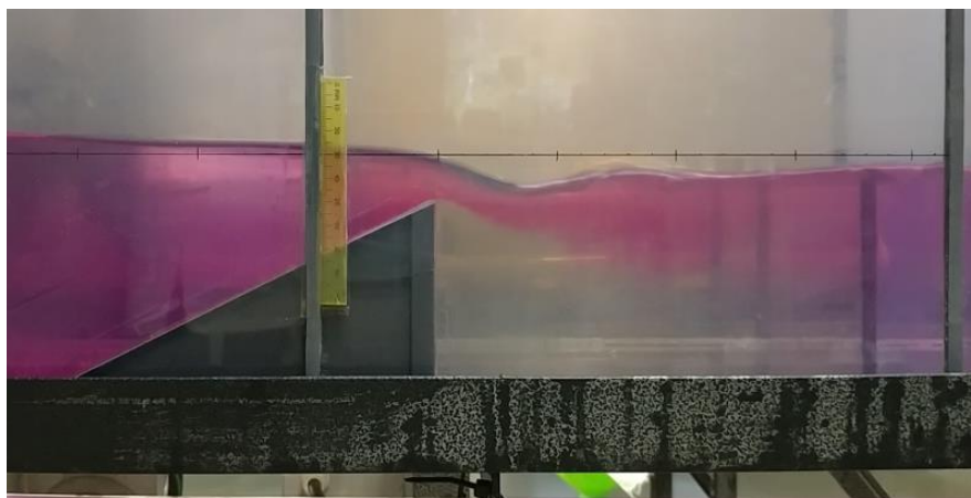
Figure 3-4: The recirculation zone after the 20 cm slope visualized using the phenolphthalein tracer
