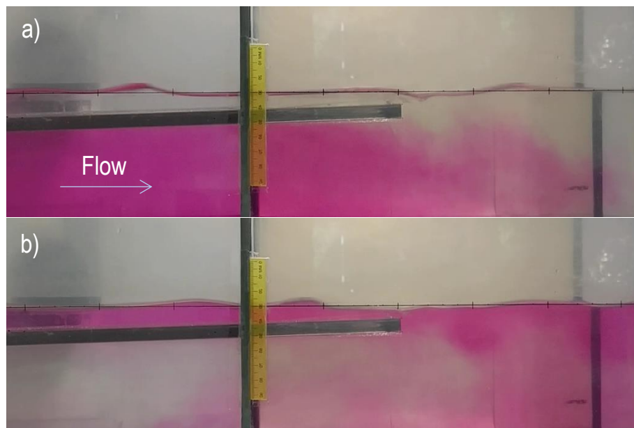
Figure 4-9: Flow pattern over slope PW visualized using phenolphthalein. The fluid on the slope slows down due to friction, as seen in a), where the tracer has not reached the end of the slope compared to the bulk fluid. b) The mixing layer after the slope due to the convergence of two streams with different velocities.
