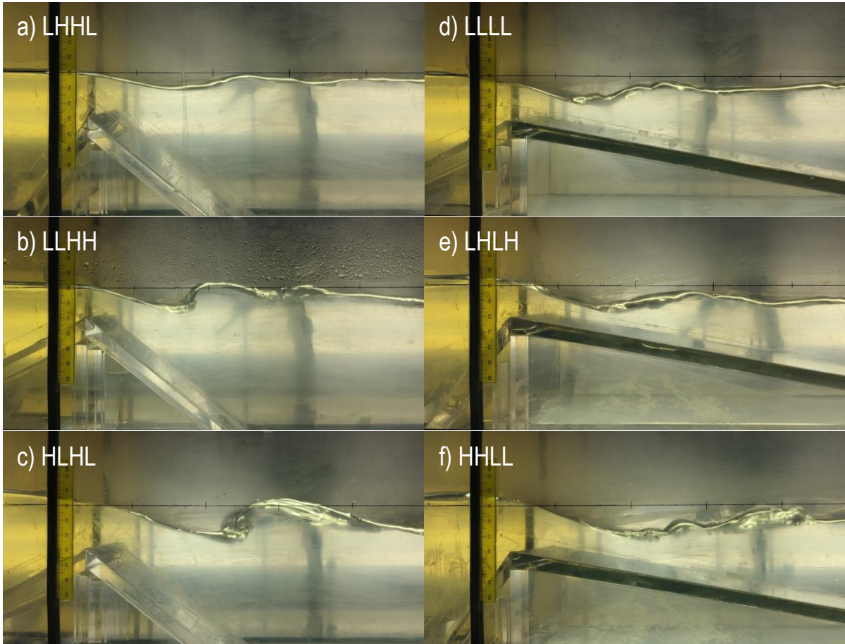
Figure 4-10: Examples of two different wave flow patterns observed for different slope configurations. a-c) depict the undular jump, for slope configuration LHHL, LLHH and HLHL respectively. d-f) depict a pattern closer to a surface jump, for slope configuration LLLL, LHLH and HHLL respectively.
