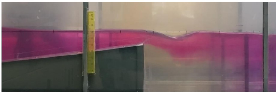
Figure 4-3: Recirculation zone observed after the 80 cm slope. Both the 20cm and 80 cm slopes resulted in a recirculation zone of a similar size, which contradicts what was stated by Burke (2016)
