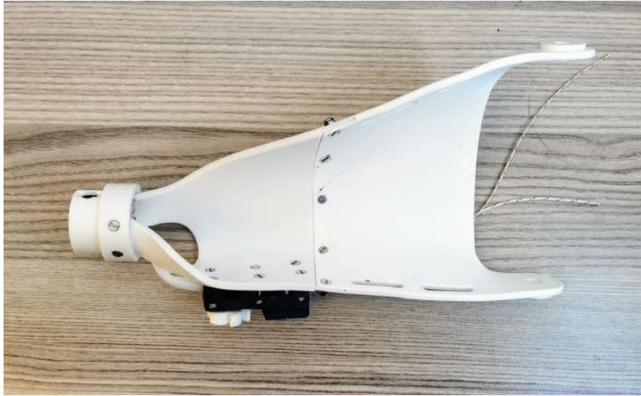
Figure 4.16: 3D printed, assembled, and moulded forearm cuff; featuring AS cable-lock mechanism.
