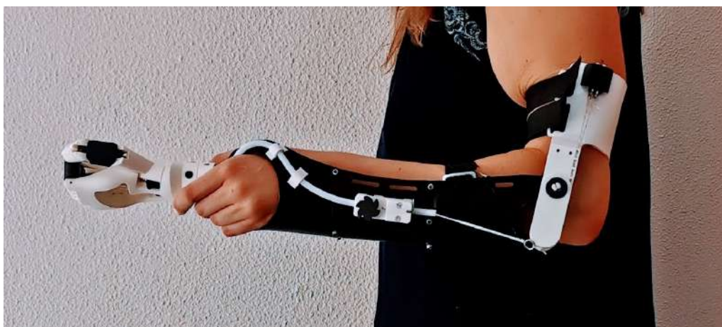
Figure 4.18: Designed bypass socket that enables non-amputee participants to use the ADL arm.
