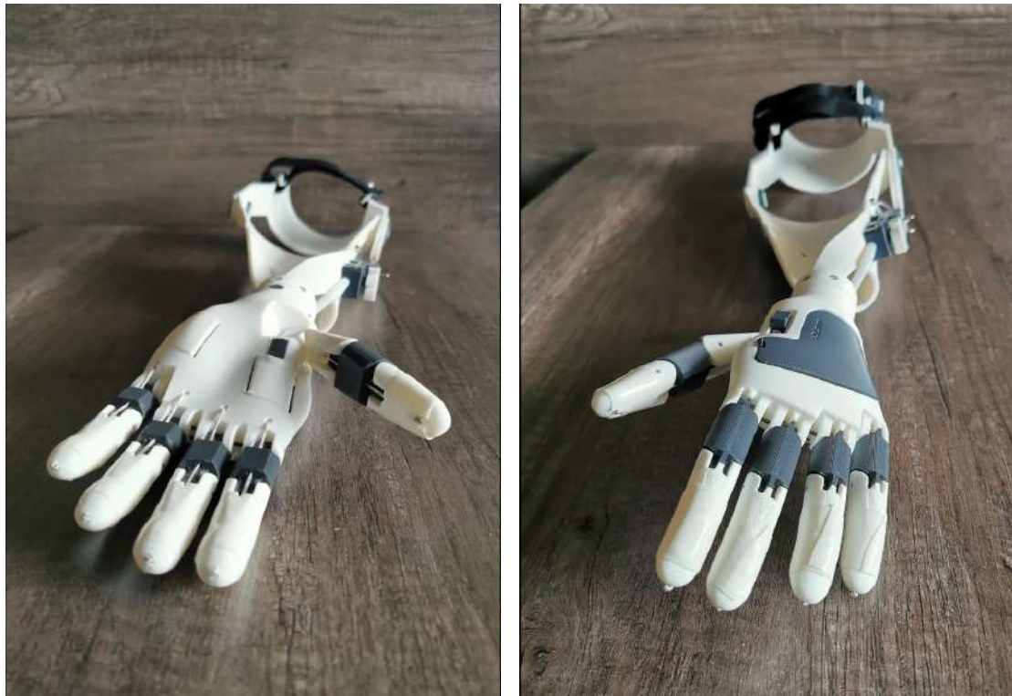
Figure 4.23: Close up of the ADL arm V2, viewed proximally, showing the palmar side (left) and the dorsal side (right) of the hand TD.
