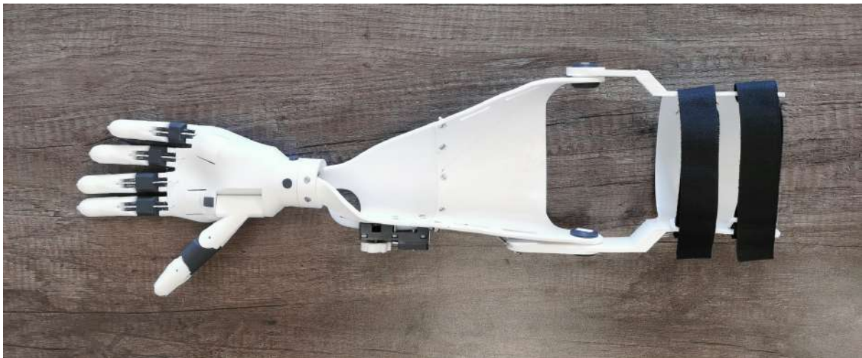
Figure 4.21: Top view of the ADL arm V2, showing the wrist in the supinated position, the thumb in full adduction, and the Velcro straps of the suspension mechanism.
