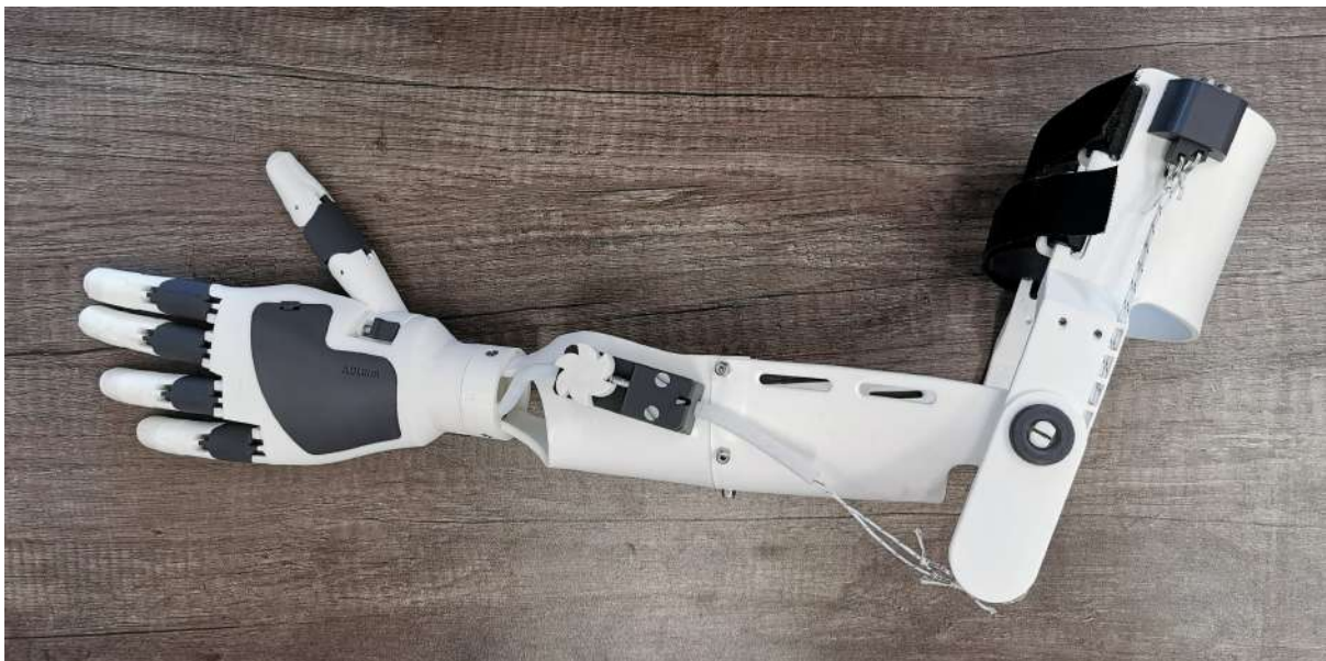
Figure 4.22: Side view of the ADL arm V2, showing the tensioning mechanism on the humeral cuff, the elbow actuation mechanism, the cable-lock mechanism on the forearm cuff, the wrist in the neutral position, and the thumb fully adducted.
