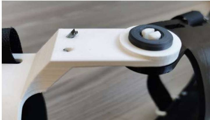
Figure 4.19: Reinforcement of the elbow struts to overcome the inherent weakness of 3D printed parts between layers.
