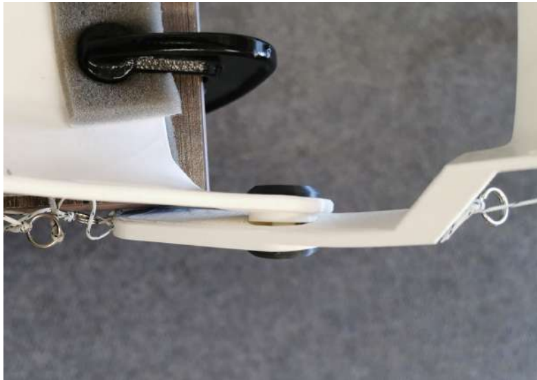
Figure 6.3: The stopping condition is where the elbow mechanism (viewed here from above) shows signs of stress but remains intact.
