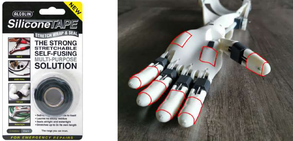
Figure 4.20: Silicone tape (outlined in red) used on the fingertips and palm to increase friction with the object being grasped, resulting in a more secure grip.
