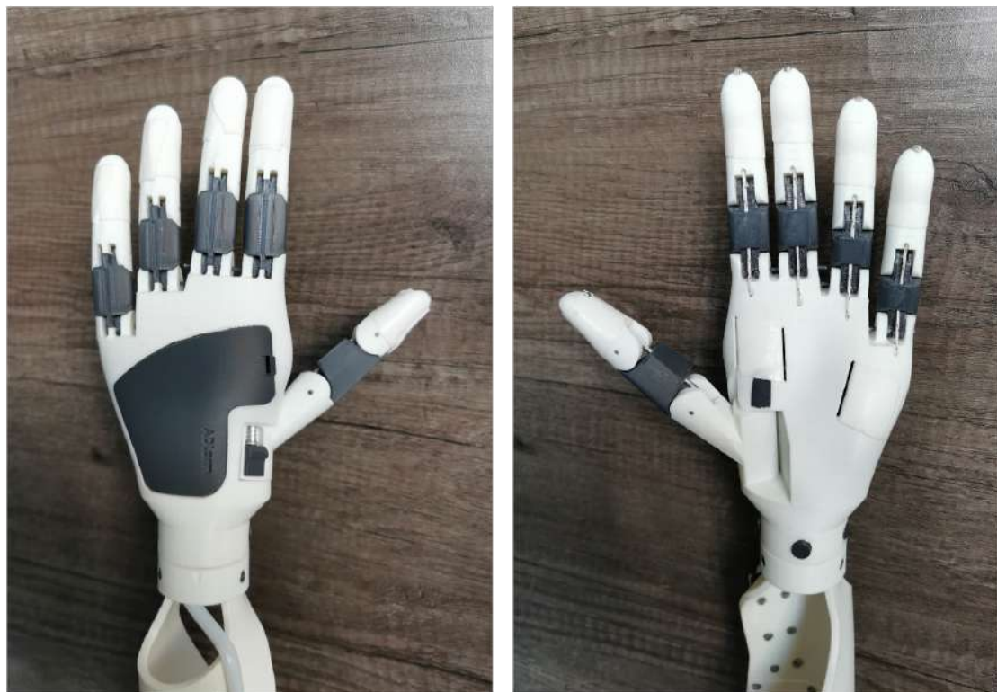
Figure 4.24: Hand TD of the ADL arm V2, showing the swivel thumb, rotating wrist, digits with actuation cords, and white silicon grip elements on the digits and palm.
