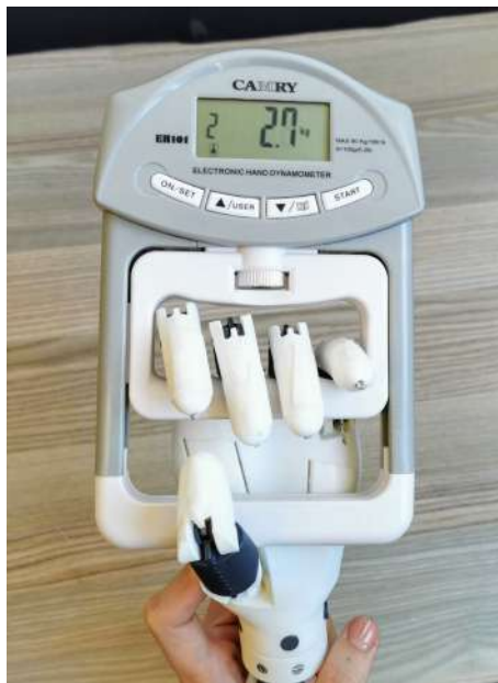
Figure 6.1: Experimental setup for measuring the grip force of the TD using a hand grip dynamometer.
