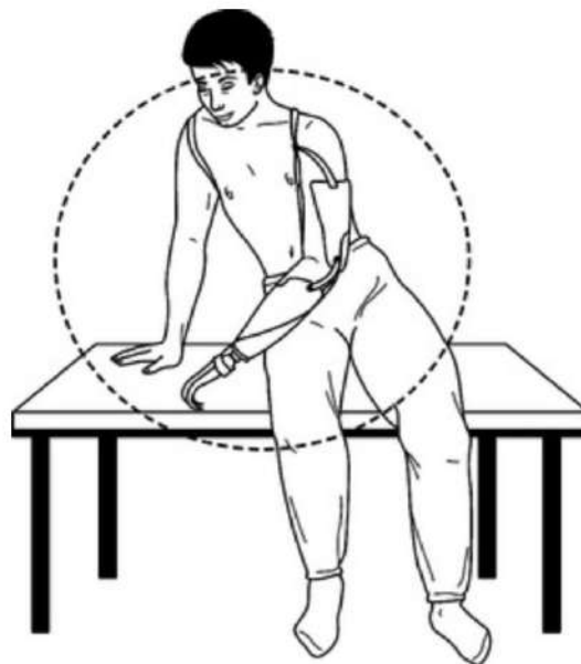
Figure 2.10: The functional work envelope of a typical body-powered prosthesis.
