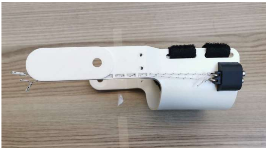
Figure 4.17: 3D printed and moulded humeral cuff; featuring AS tensioning mechanism.
