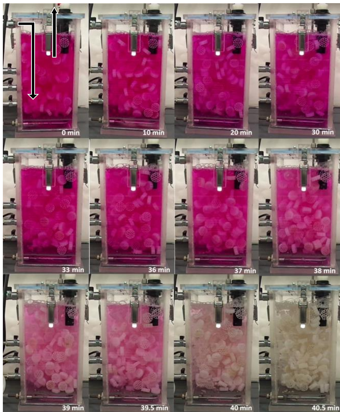
Figure 6-7: Time lapse showing the mixing profile in the MBBR at a 24 hour retention time and aeration rate of 3 L/min.
