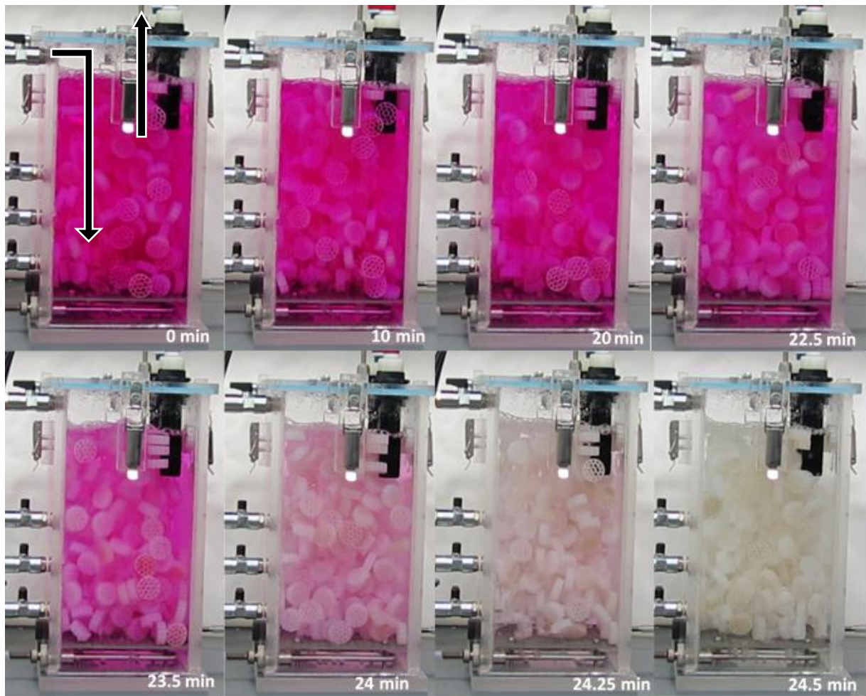
Figure 6-8: Time lapse showing the mixing profile in the MBBR at a 12 hour retention time and aeration rate of 3 L/min.
