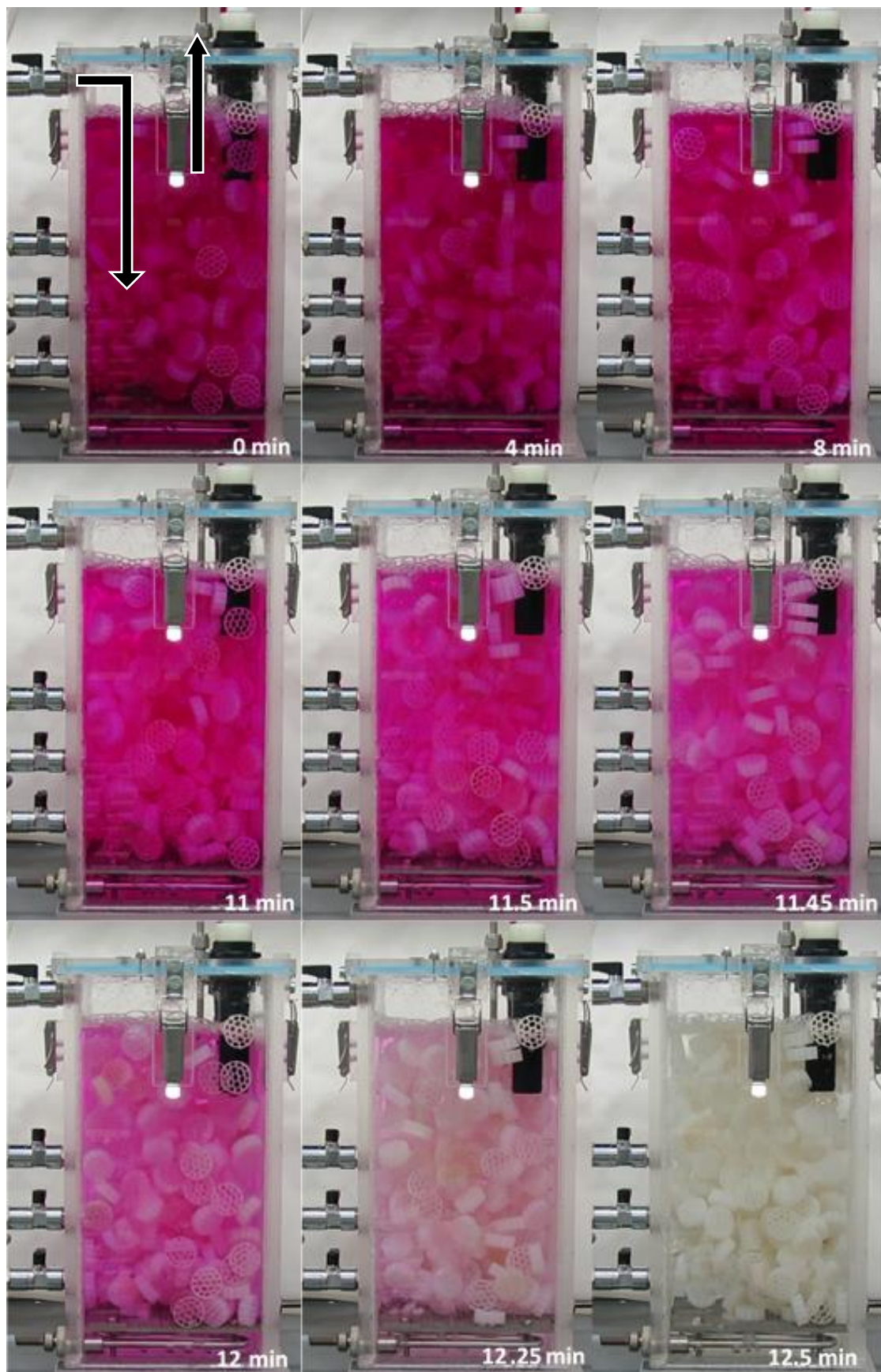
Figure 6-9: Time lapse showing the mixing profile in the MBBR at a 6 hour retention time and aeration rate of 3 L/min
