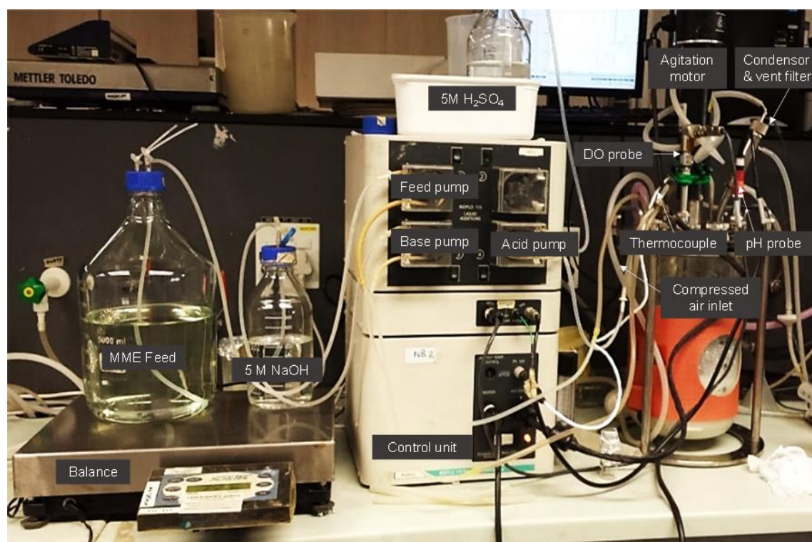
Figure 4-2: Setup of Bioflo 110 New Brunswick bioreactor for fed-batch cultivations
