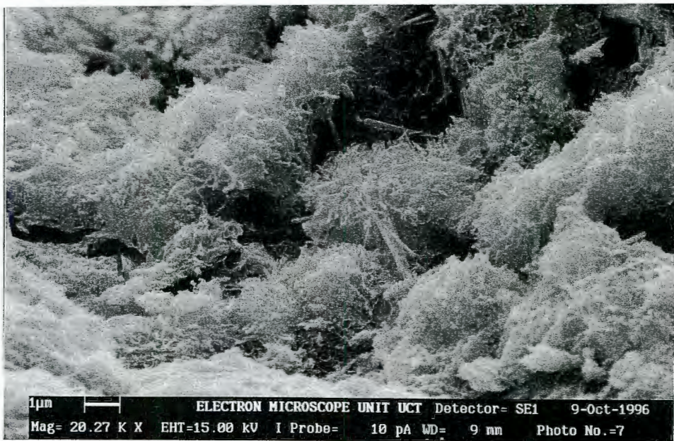
Figure 4-4 - Hardened Cement Paste after 28 Days Curing
