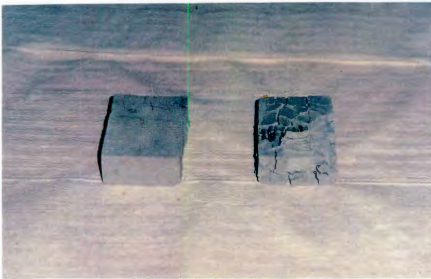
Photograph 7-1 - Unleached and Leached Solidified FeCr Dust (Both after Drying)
