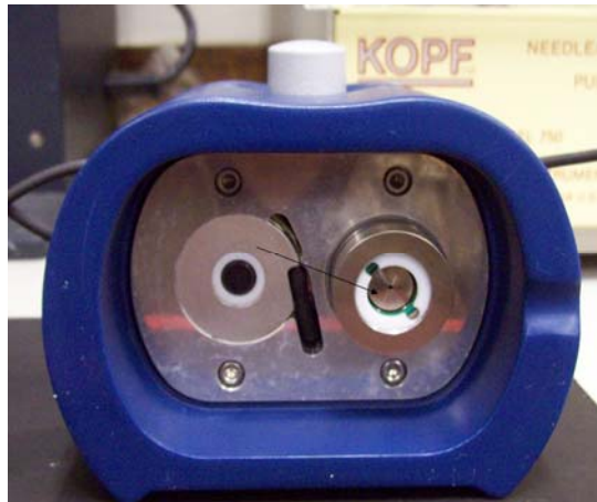
Figure 3.2. The Q -sense chamber where the sensor crystal is mounted (shown by an arrow)
