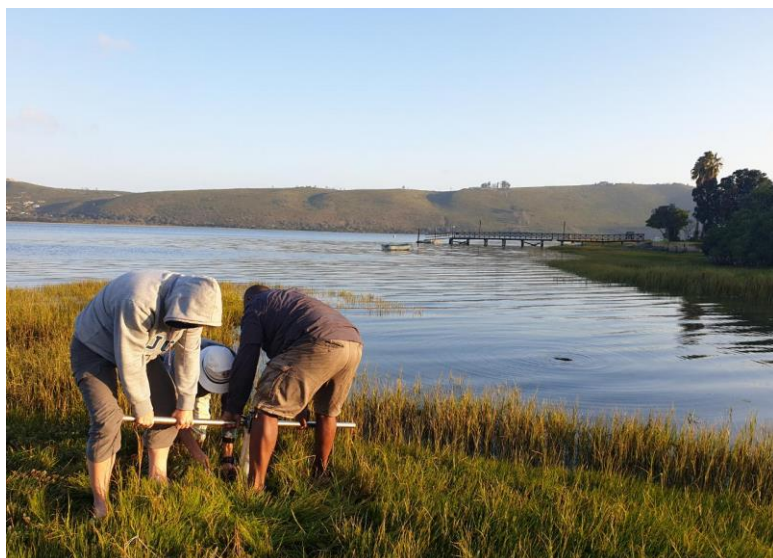
Figure 8. Manual coring device, along with adjustable lever. Figure 9. Cores were labelled and sealed.
