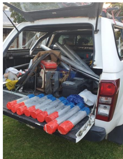
Figure 8. Manual coring device, along with adjustable lever. Figure 9. Cores were labelled and sealed.
