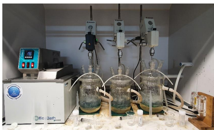
Figure 3.12: Experimental set up of batch stirred tank reactors
