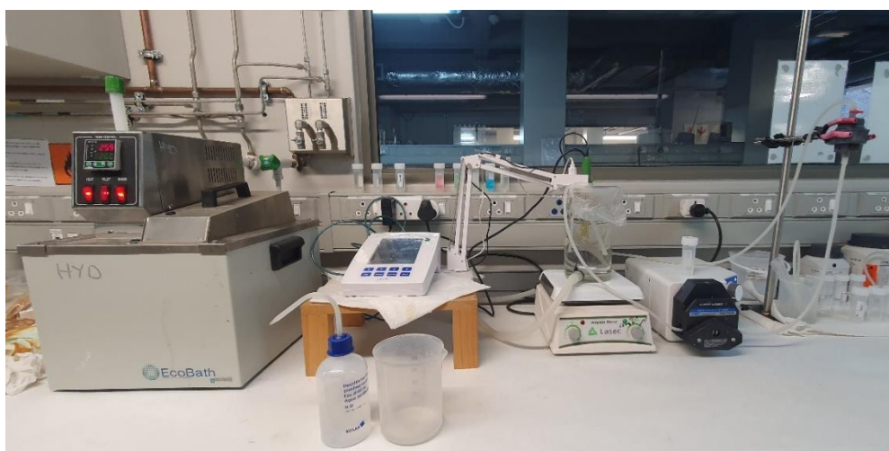
Figure 3.15: Experimental set up for ion exchange experimentation
