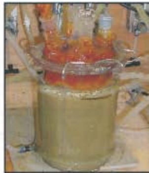
Figure 4.6: Chalcopyrite bioleaching STR showing extensive jarosite present in the reactor after 30 h. STR operated at a 3% mineral loading and an impeller tip speed of 1.97 m s -1 .
