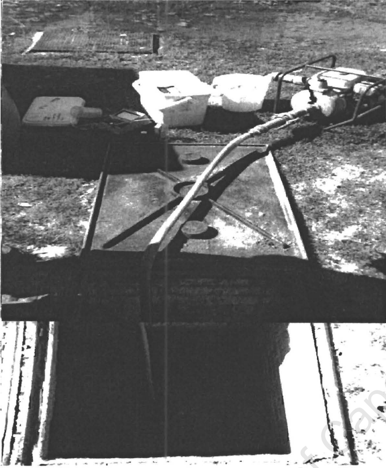
Figure 3.2: A complete set-up of the borehole sampling equipment.
