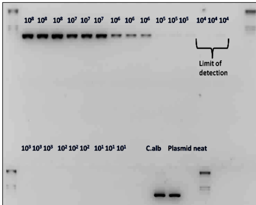
Figure 6. Agarose gel electrophoresis of the limit of detection experiments using a control plasmid containing the ITS1 – 2 PCR amplicon from C. albicans , serially diluted ten-fold from 10^8 – 10^1 target
