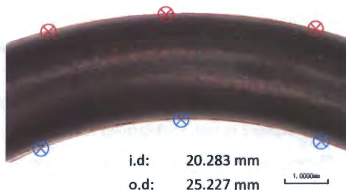
Figure 3.1: Microscope image of a magnified O-ring indicating the selection of the three points required to obtain the inner (i.d.) or outer (o.d.) diameter
