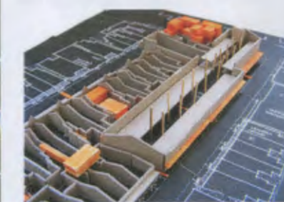
Creating a double volume atrium space to bring light down the centre of the building.
