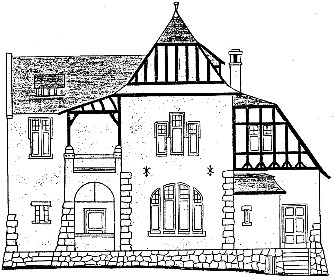
Rukwied: Bezirksamtshaus, Lüderitzbucht, 1908. Preference is given to narrow vertical windows, placed rhythmically to accentuate the asymmetrical proportions of the building.
