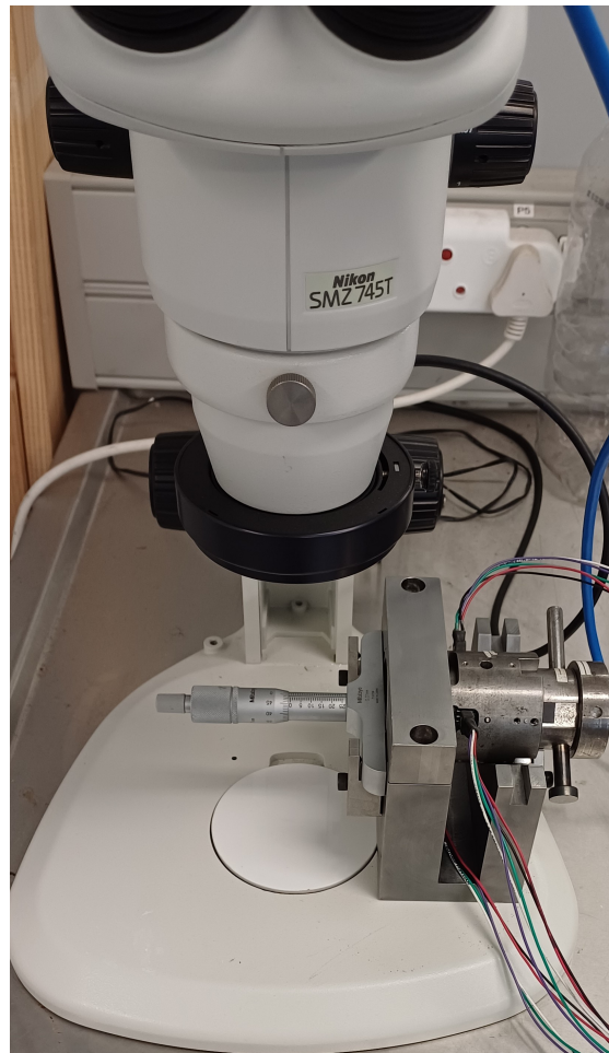
Figure 3.4 The sub-press and mounting fixture placed under the microscope.
