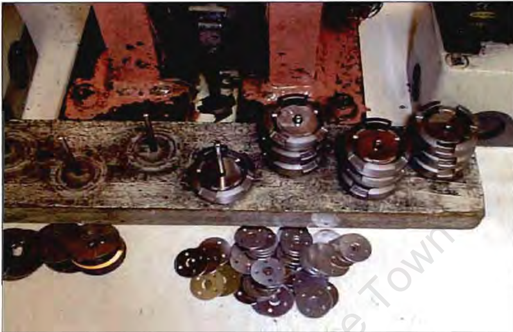
Figure 2.4: The subassembly palette. Thirty subassemblies can be done at a time on these palettes.
