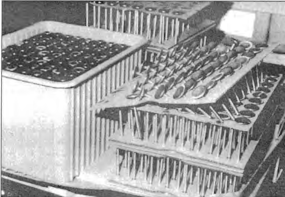
Figure 3.6: Two examples of storage methods of cylinder head valves. The picture shows the problems with the storage method on the right hand side.
