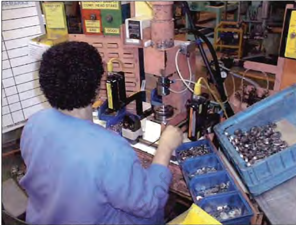
Figure 2.3: The compression head valve assembly cell.
