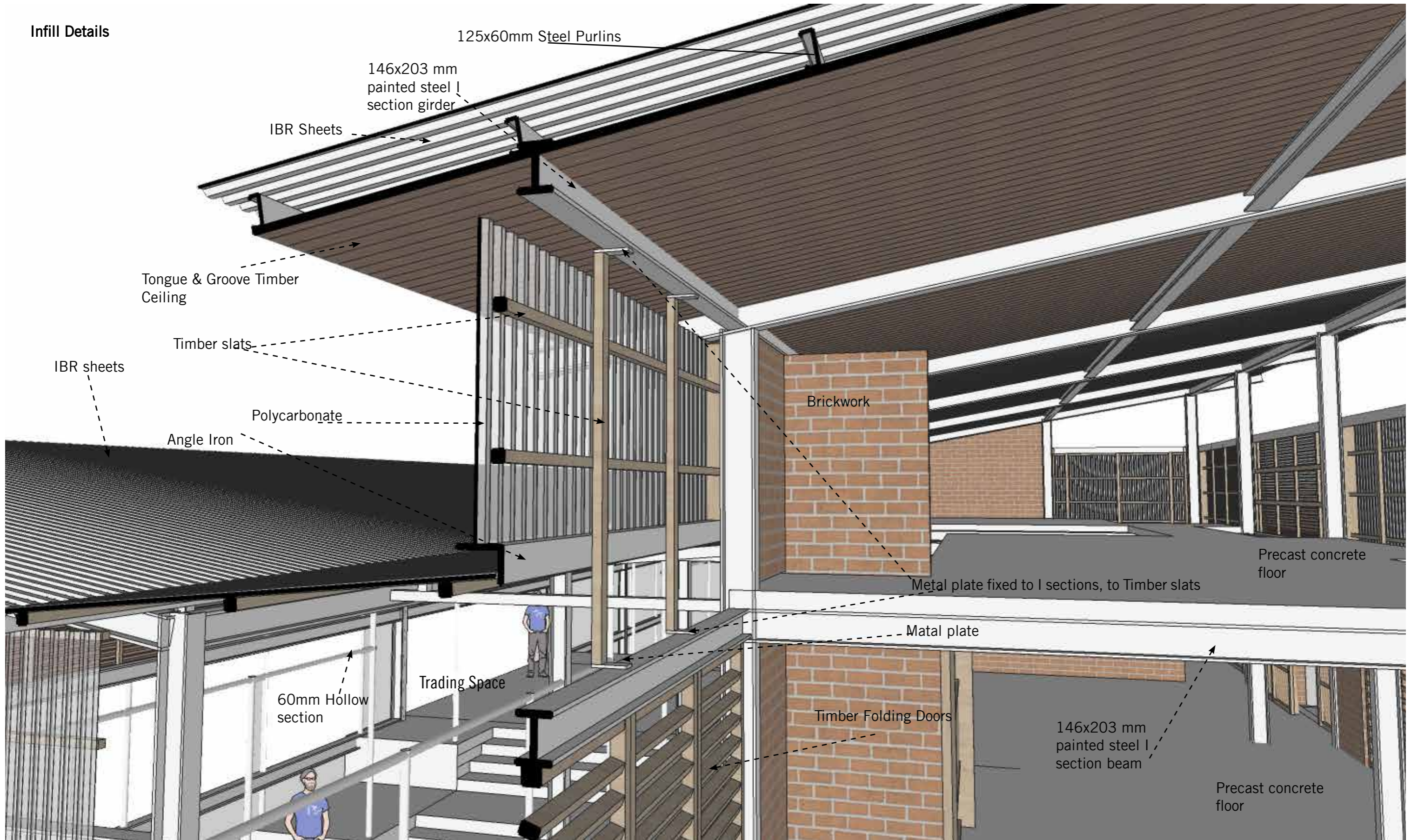
Section perspective showing infill and structural assembly.
