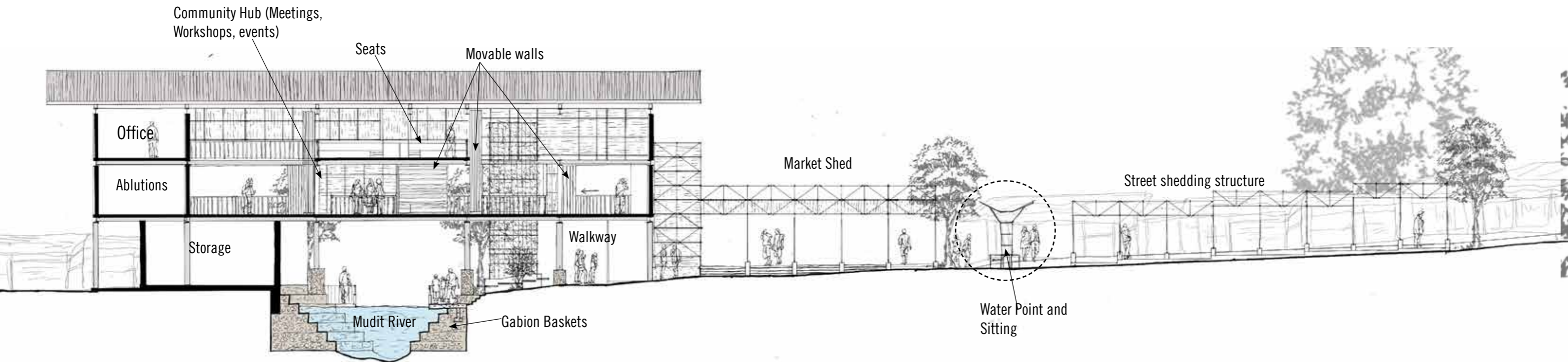
Section A: Through Mudi River, Community Hub, Recreation Space, and the proposed scaffolding steel structure market sheds.
