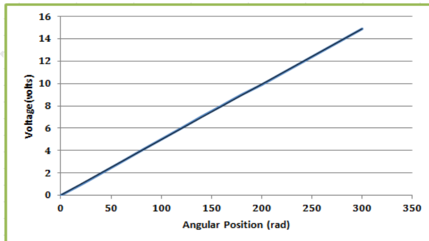
Figure C1: The relationship between angular displacement and output voltage.
