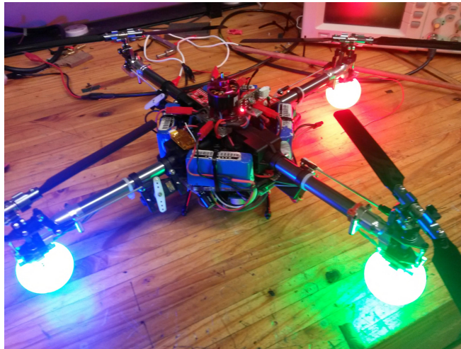
Figure 2.14: First iteration of active markers on quadcopter. The motion capture system was configured to identify dominant blue, red, and green features within a camera image.
