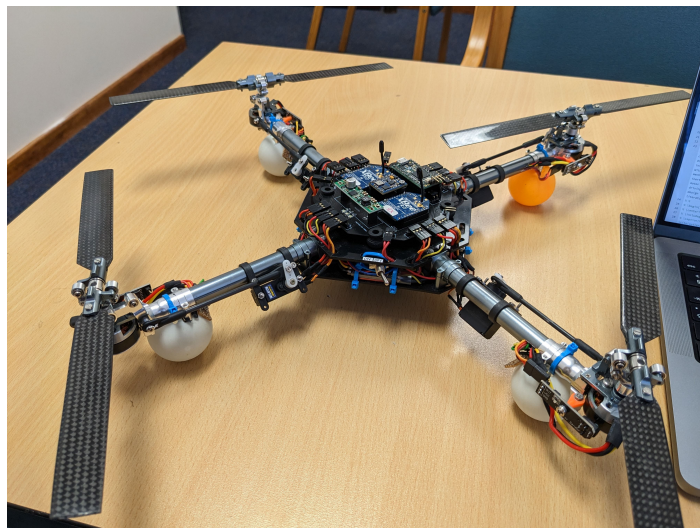
Figure 1.1: Fully assembled variable-pitch quadcopter.
