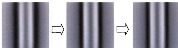
Figure 2.4.1: The three averages produced during the initial centring of the helices in the x-dimension. Noticeably the average becomes more defined and the x-shift values begin to remain the same after approximately three alignment steps.
