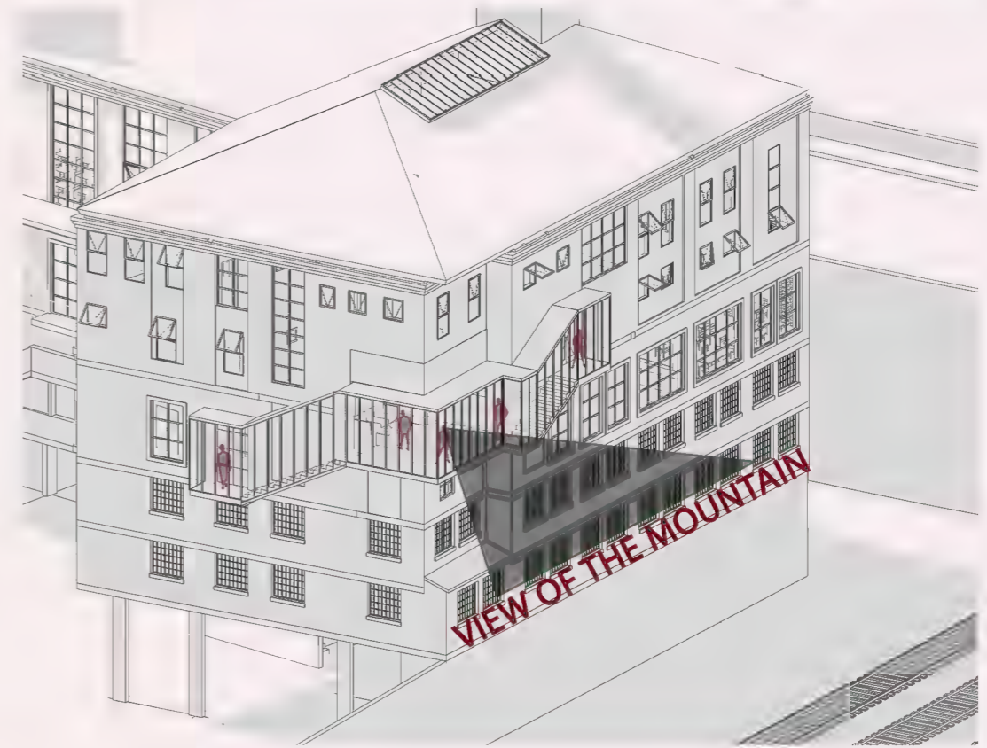
RECENT RENOVATION OF THE ORIGINAL BUILDING | CREATING NEW EXTRUDED STAIRCASE
