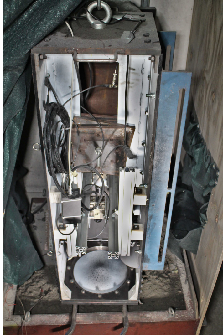
Figure 3.13: The new pendulum with attachments added and hanging as a vertical pendulum
