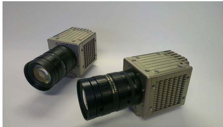
Figure 3.18: Photograph of the two IDT NRS4 cameras that were built into the pendulum to capture the images used for DIC.
