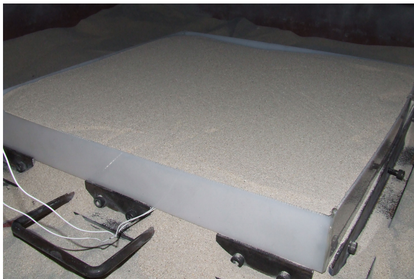
Figure 3.16: HDPE frame filled with sand to create the desired depth of burial
