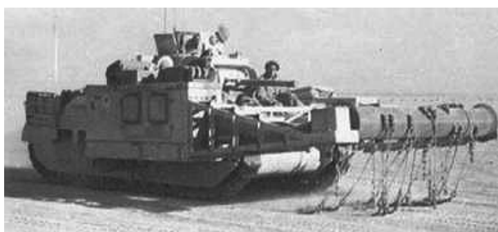
Figure 2.5: Flail truck used to actively detonate landmines in the field [23]
