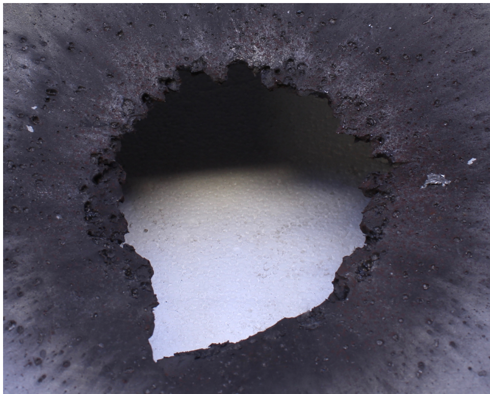
Figure 4.13: A close up photograph of the shrapnel damage resulting from the exposure of a plate to an encased charge in air. Total distance 100 mm.
