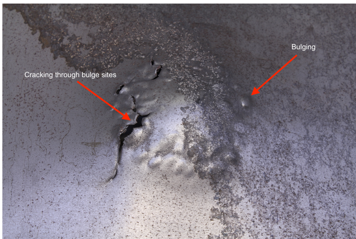
Figure 4.20: A photograph of the rear side of a plate exposed to an encased charge buried under 1 mm of sand, indicating bulging and cracking. 91.34 Ns impulse.
