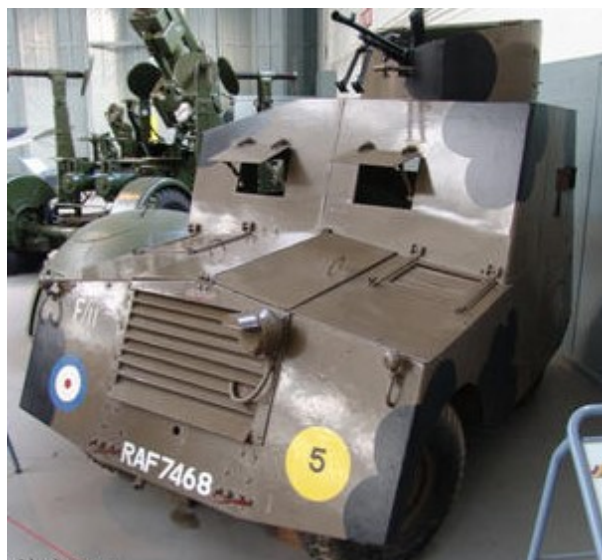
Figure 2.4: Standard Beaverette Light Armoured Car - light steel plates fitted to a standard truck [29]
