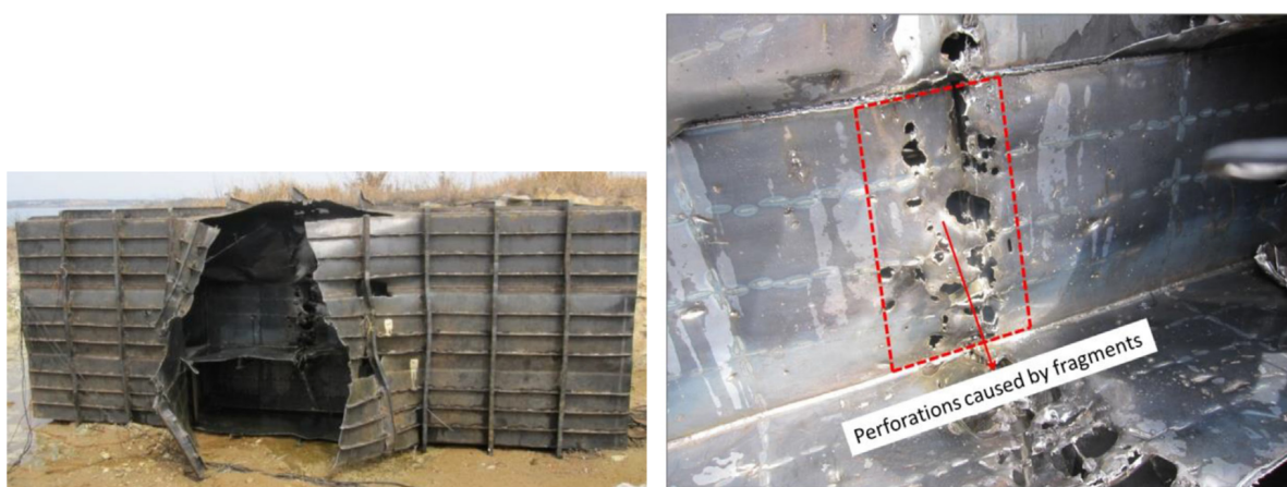
(a) Large deformations and rupture of stiffened plates et al. [80]. (b) Perforation damage observed adjacent to charge location [80].
