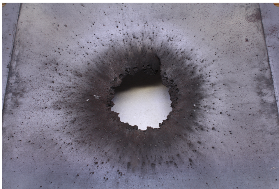
Figure 4.12: A photograph of the capping failure and shrapnel damage resulting from the exposure of a plate to an encased charge in air at 100 mm total distance. 75.52 Ns impulse.
