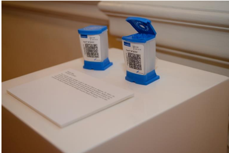
Image 8: Exhibition display of the GeneXpert MTB/RIF. TB is diagnosed in this plastic cartridge in two hours. Inside the cartridge, bacterial DNA from a sample is extracted and copied in order to detect the presence of TB as well as resistance to the TB drug Rifampicin. Photo courtesy of Cliff Shain.
