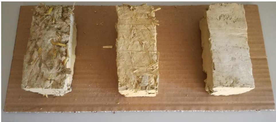
Figure 30: Initial Experiment using cardboard moulds. Straw, Clay and Cement (Left), Clay and Straw (Middle) and Clay and Cement (Right) (Author, 2023).
