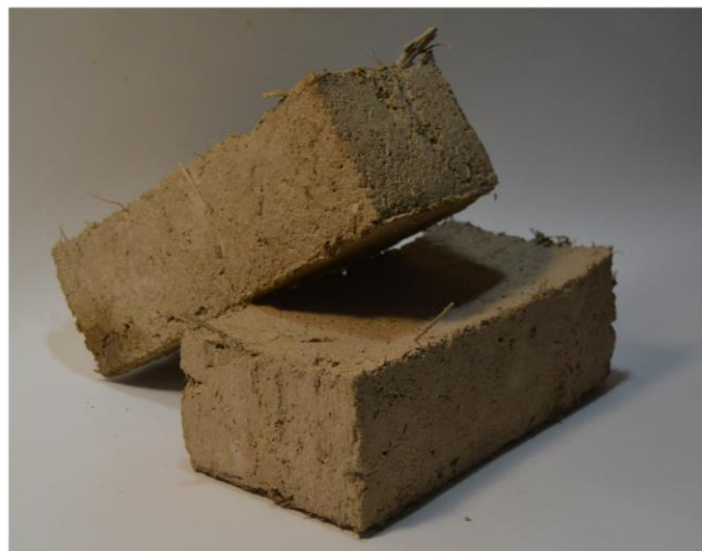
Figure 31: Documenting the Adobe Brick Making process using Clay, Straw, Sand and Horse manure (Author, 2023).
