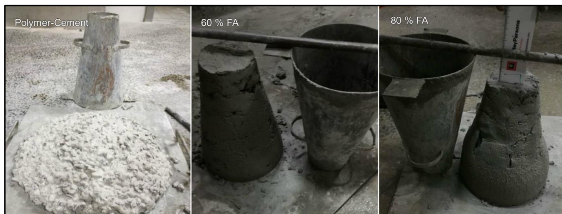
Figure 4-6: Repair material slumps
