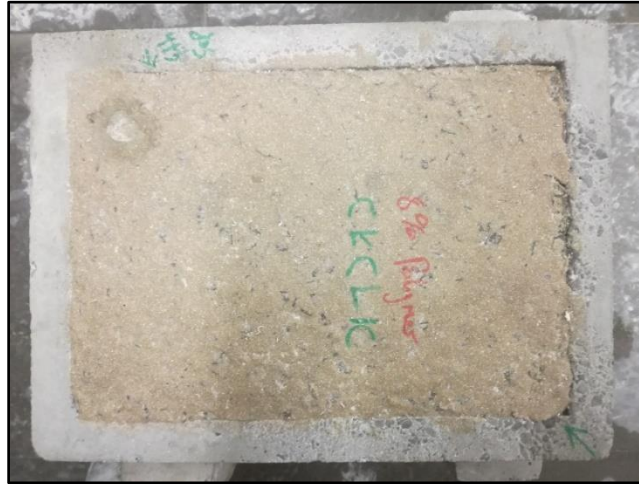
Figure 4-22: 8% polymer concrete patch repair after cyclic wetting and drying
