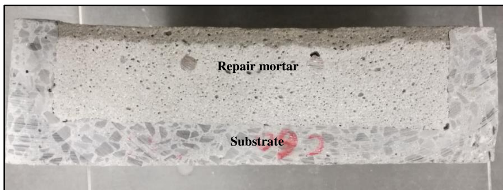
Figure 4-21: Cross-section of 60% FA patch repair after cyclic wetting and drying
