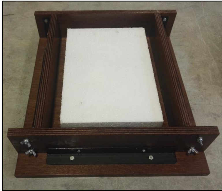
Figure 3-20: Wooden mould used to cast substrate concrete slabs (with styrofoam insert to create the cavity for mortar application)
