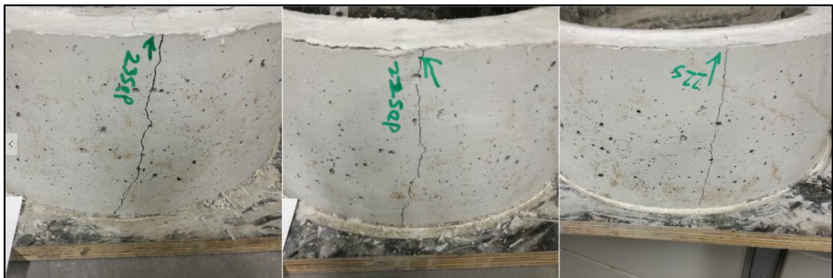
Figure 4-46: Crack distribution on 60% FA rings
