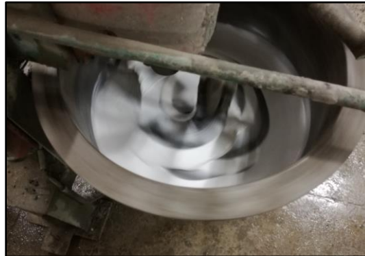
Figure 3-18: Mechanically mixing polymer with water
