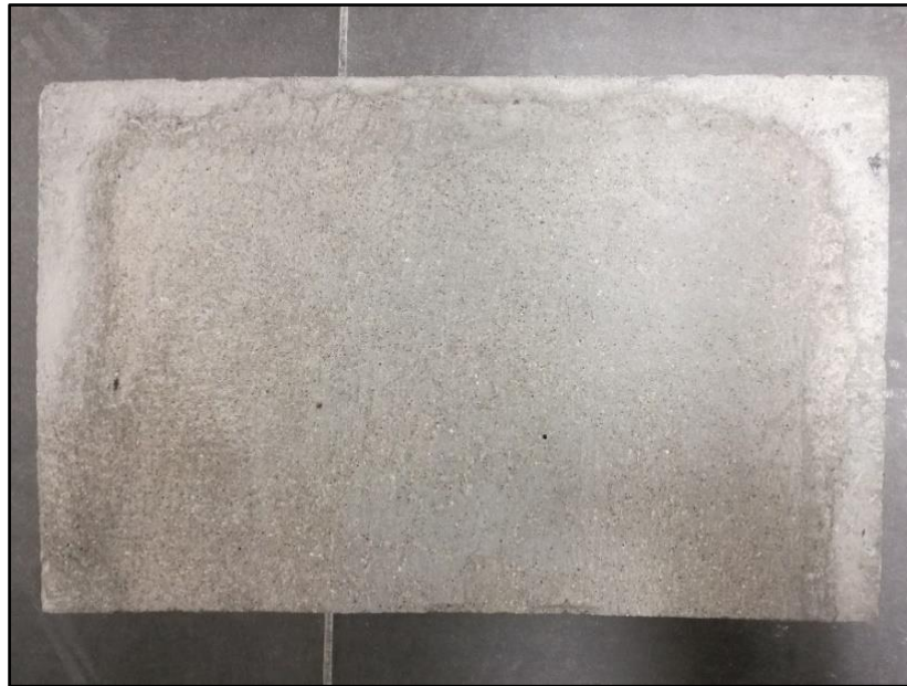
Figure 4-20: 60% FA patch repair after cyclic wetting and drying
