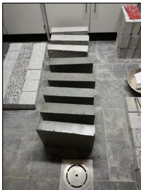
Figure 3-25: Substrate moulds left for drying in the control room
