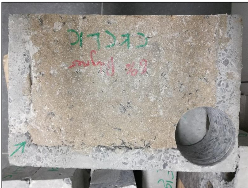
Figure 3-38: Core for SEM taken from corner of substrate mould
