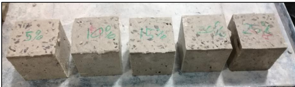
Figure 3-17: Polymer-cement concrete trial cubes (100 mm cubes)
