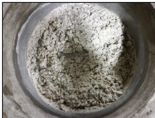
Figure 3-19: Polymer-cement concrete repair material after mixing
