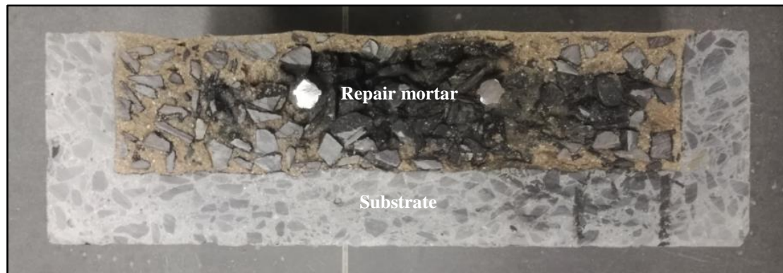
Figure 4-25: Cross-section of 9% polymer concrete patch repair after cyclic wetting and drying
