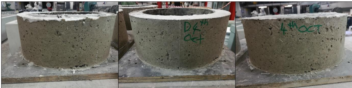
Figure 4-48: No cracking on polymer-cement concrete rings
