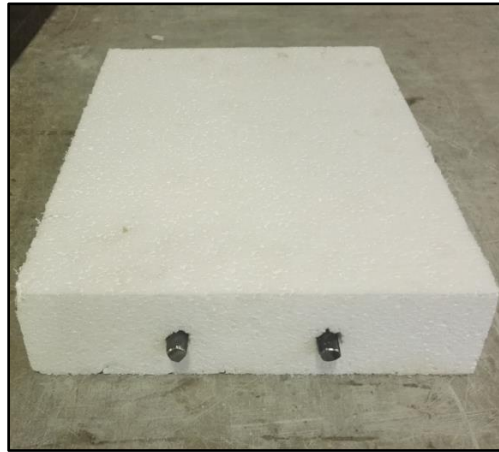
Figure 3-22: Styrofoam with embedded 10 mm diameter steel bars
