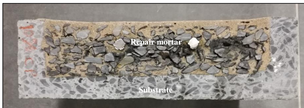
Figure 4-27: Cross-section of 10% polymer concrete patch repair after cyclic wetting and drying
