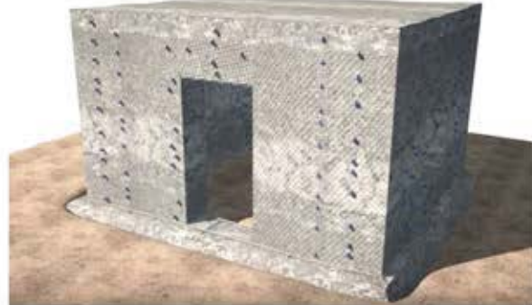
8) The roof is cast by using conventional wood shuttering with fishnet ropes over it. A concrete slab (1 part cement, 3 part sand, 3 part gravel 16mm) is cast over the fishnet ropes and a layer of fishnet is placed on top.
