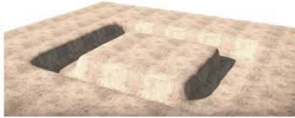
1) Foundations trench dug as per load bearing capacity of soil.
