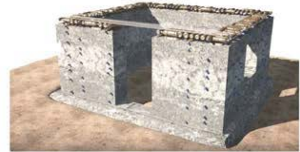
6) Windows and doors are created by pulling the fishnet rope in high tension, 60 cm beyond the opening.
