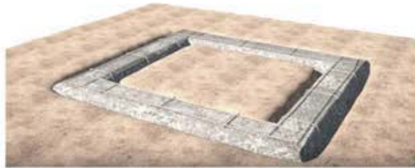
4) A mixture of 1 part cement and 6 parts sand is poured between bottles. Nylon 6 fishnet (210 denier, 3 ply, 3cm x 3cm) and fishnet ropes (Nylon 6 fishnet cut 20 squares wide & twisted to make ropes) are placed over foundation.
