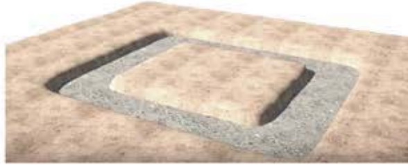
2) 15cm of PPC cement laid at base of foundation trench.
