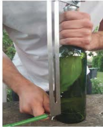
Cut clean glass bottles and split by thermal shock along the score line.
