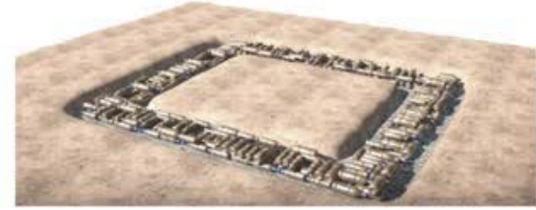
3) Bottles placed in trench at twice the width of the wall.
