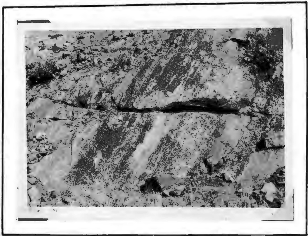
Crystals of magnetite and martite protruding from a matrix of quartz and barite.
