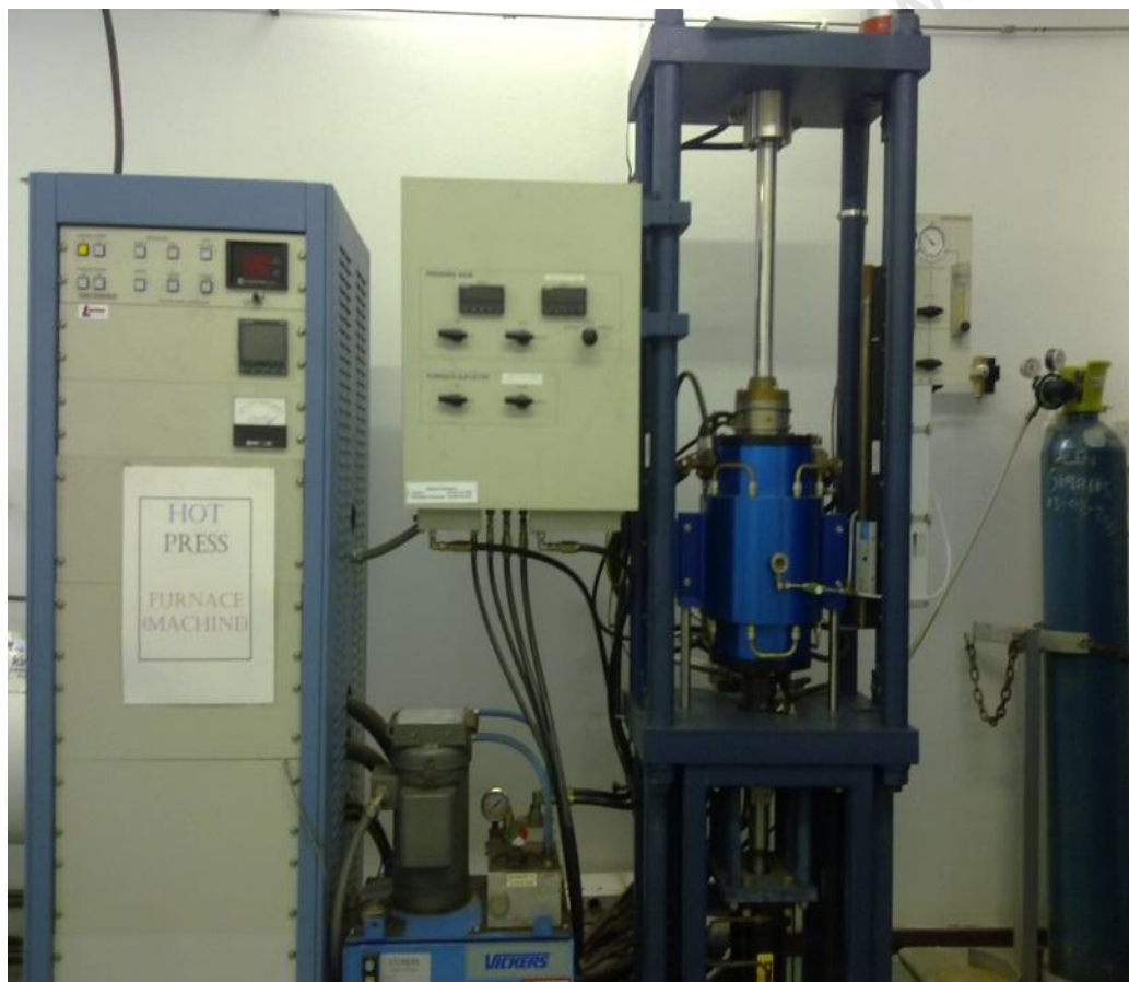
Figure 3.1: The hot-press used to sinter powders for MAX phase synthesis.
