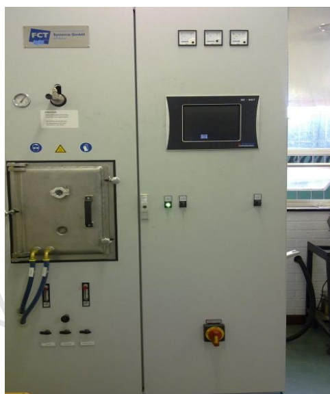
Figure 3.2: The SPS used to sinter cBN/MAX powders to synthesise the composite material.
