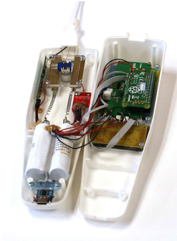
Figure 3-16 Assembled Handheld Base
