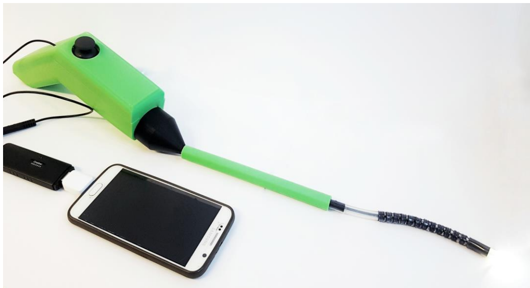
Figure 3-11 Prototype 2 Completed. The prototype improved on the previous with a smaller diameter camera, multiple bending directions and greater bending angles.
