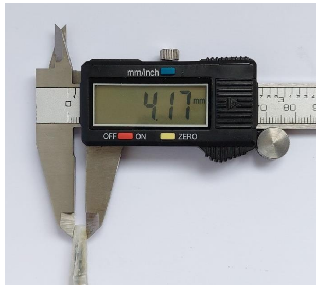
Figure 4-4 Outer Diameter with Sheath on. A digital vernier calliper was used to measure the diameter of the rod with the sheath and was approximately 4.2 mm.
