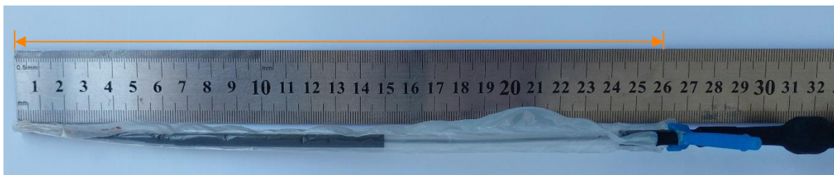
Figure 4-3 Working Length of Prototype. The working length was measured with a ruler and with the sheath on found to be 260 mm.
