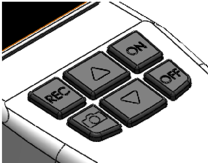
Figure 3-34 Prototype 4 Controls. The user is able to control bending up or down, record images and videos, and switch the device on and off.
