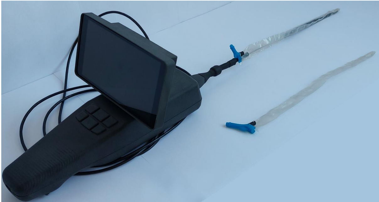
Figure 4-44 Hysteroscopy System and Disposable Sheath. The newly developed hysteroscopy system and disposable sheath accessory to be used in the testing.
