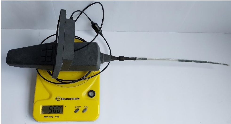
Figure 4-2 Prototype Weight. The entire prototype was weighed on a scale and found to weigh 500 g.
