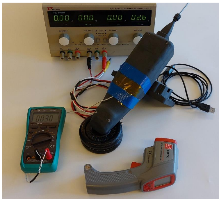
Figure 4-40 Thermal Analysis Validation Testing Setup. The setup consisted of a thermocouple fixed to a spot on the enclosure shown in the simulation to reach
