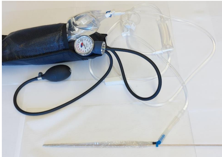
Figure 4-13 Distention Media Channel Pressure Test Setup. The pressure cuff was using to raise the pressure of the saline bag to 210 mmHg and connected to the distention media channel of the sheath.
