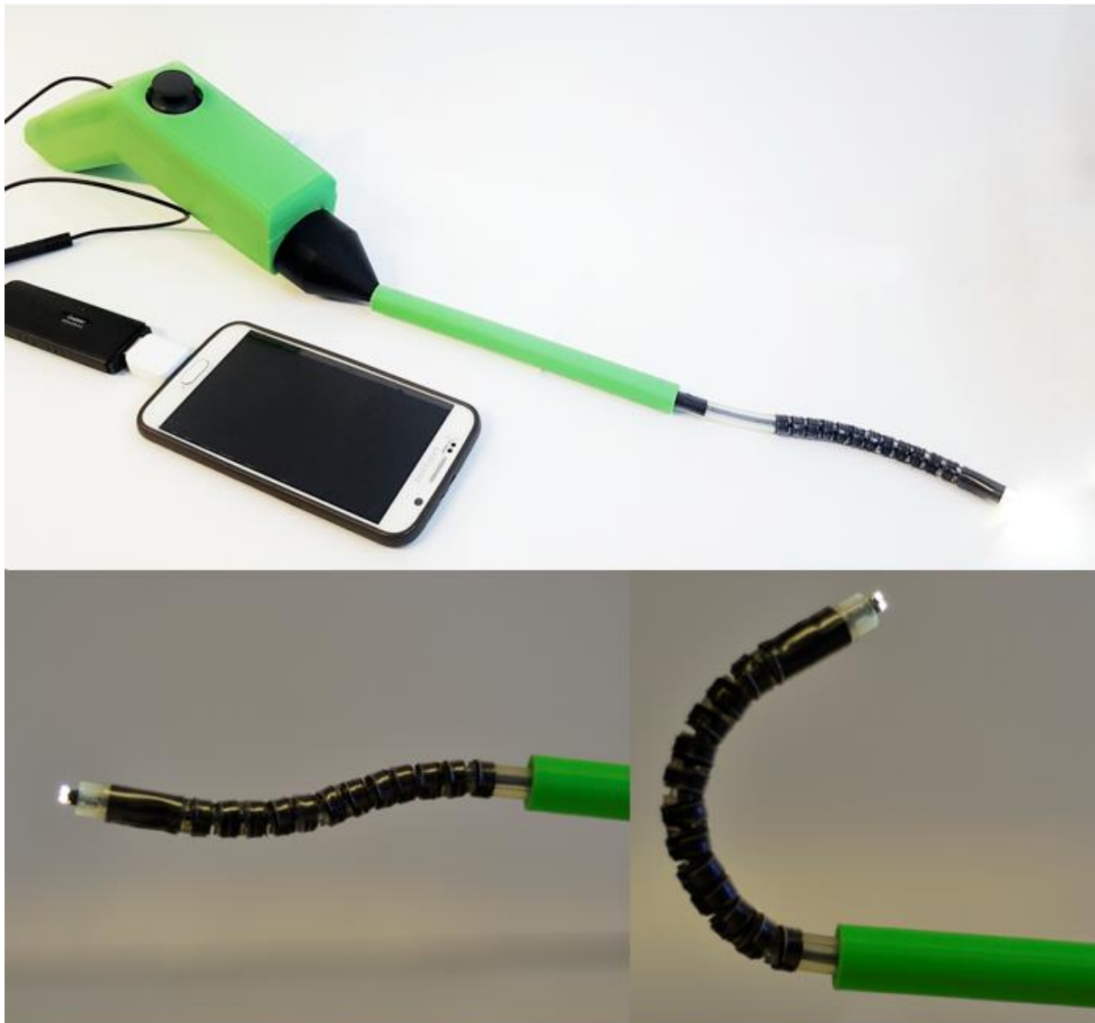
Figure B.2 Prototype 2 - Multiple Directional Bending
