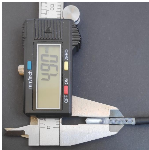
Figure 3-20 Camera Insertion Rod Diameter. A digital vernier calliper was used to measure the rod diameter of 4.90 mm.
