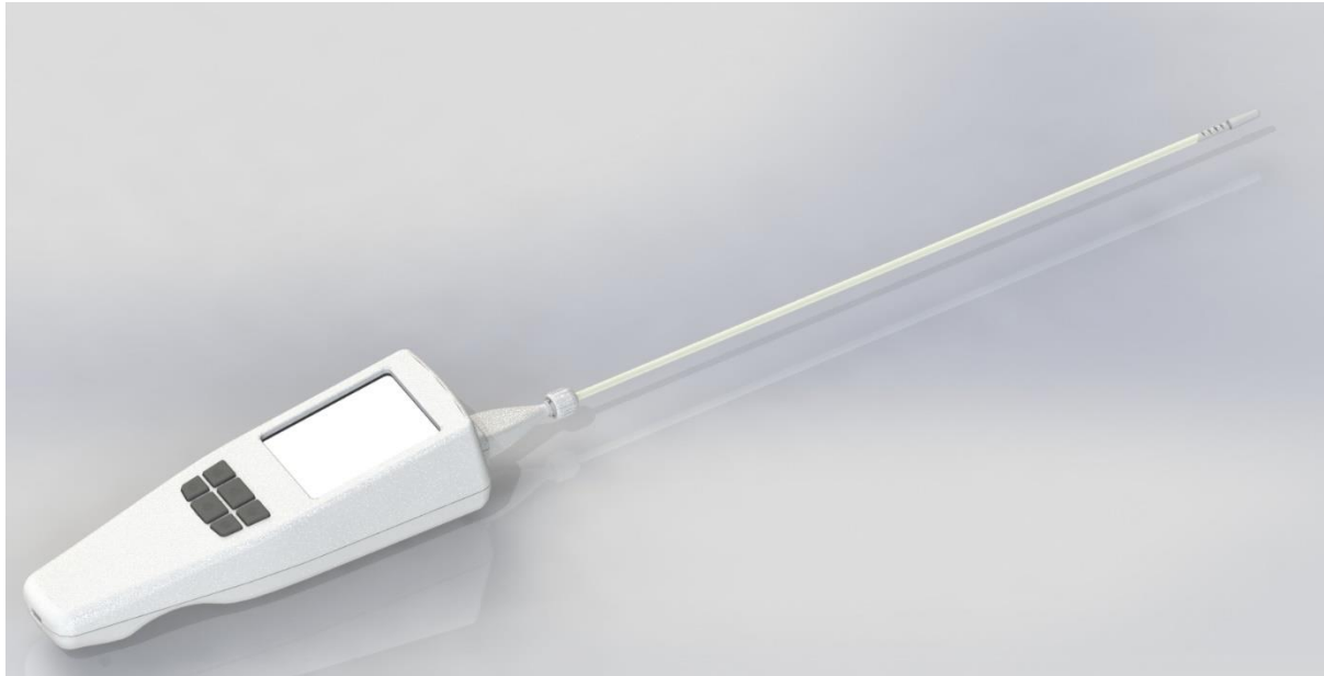
Figure 3-12 Prototype 3 Concept. Prototype 3 included an integrated screen and improved camera insertion rod design to reduce the size.
