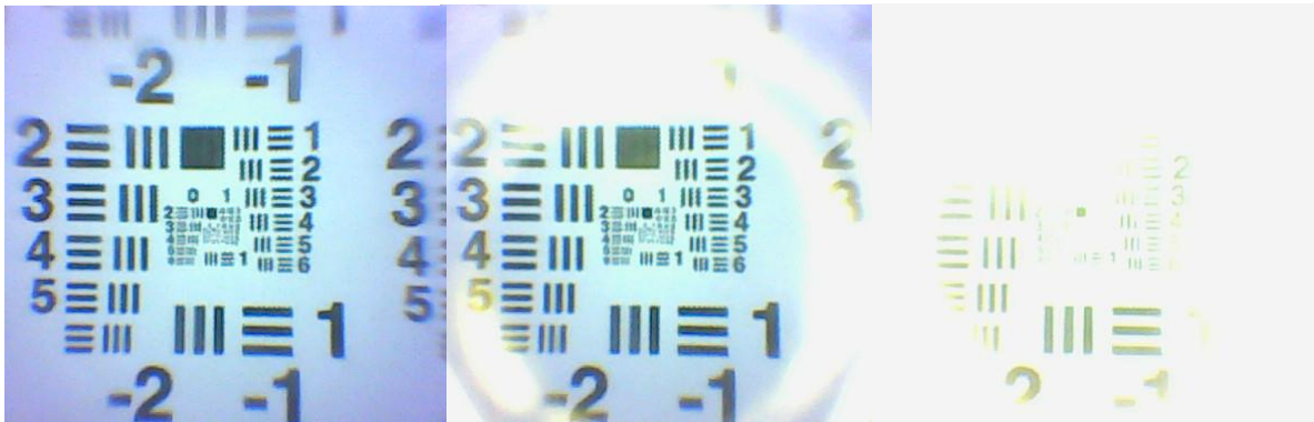
Figure 3-25 Visual Clarity at Increasing Brightness through Sheath. The sheath reduced the visibility due to the LED light reflecting back as the brightness increased.
