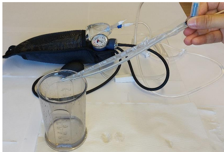
Figure 4-14 Distention Media Channel Flow. The distention medial channel was tested by allowing the saline to flow through while connected to the pressure cuff.
