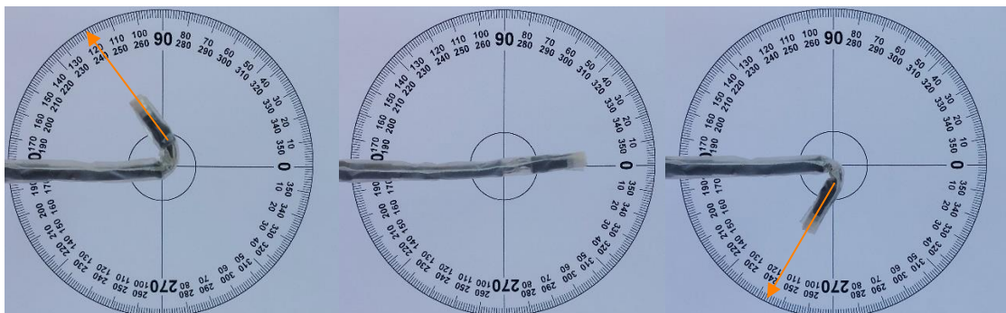
Figure 4-5 Bending Angles of Prototype. The bending angle was measured with a 360° protractor and was able to bend 120° up and 116° down.
