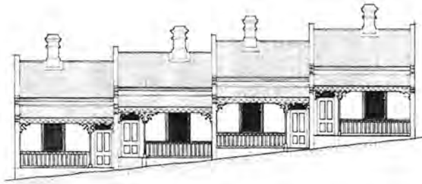
PITCHED ROOF STRAIGHT GABLES & CONTINUOUS STOEPS STEPPING DOWN TO SLOPE OF STREET
