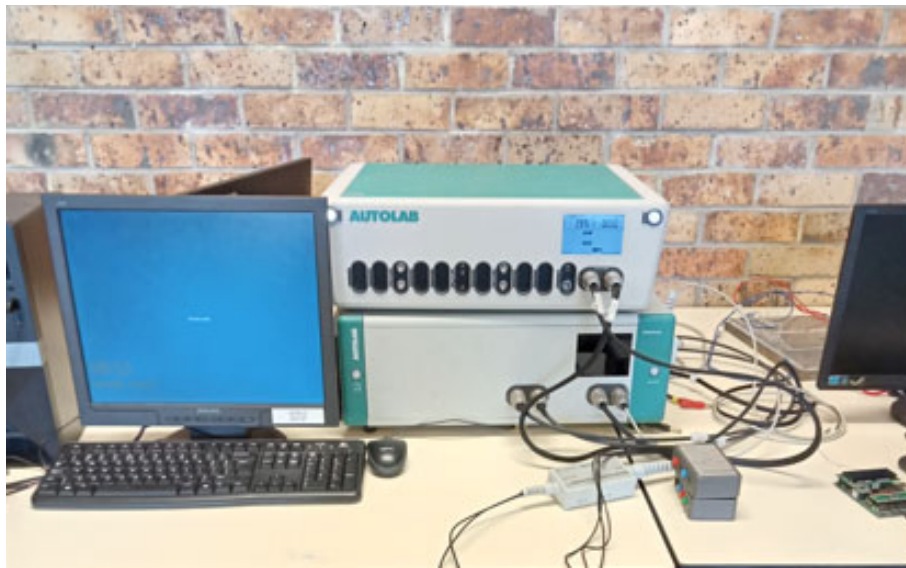
Figure 10.1 AUTOLABPGSTAT302N frequency response analyser
