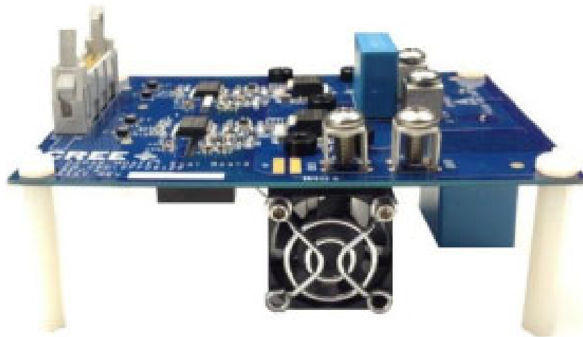
Figure 10.5 CRD-5FF0912P, SiC MOSFET High-Frequency Evaluation Board for 7L D2PAK side view.
