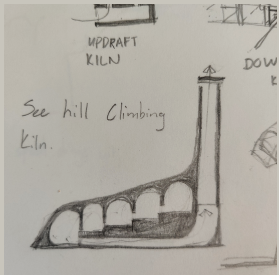
Figure 96: Hill climbing kiln design
