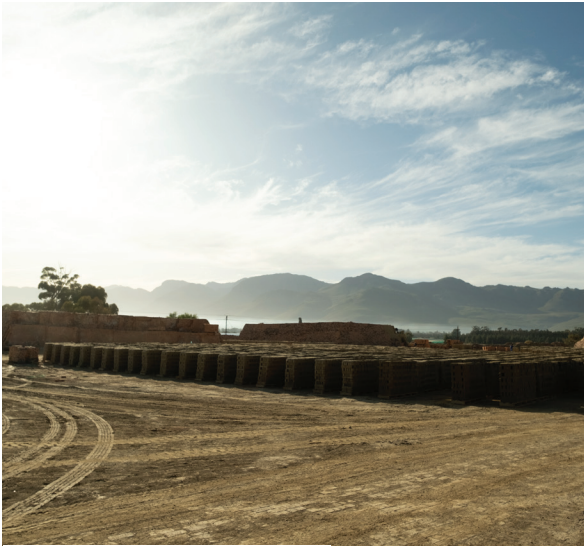
Figure 23: Green bricks drying
