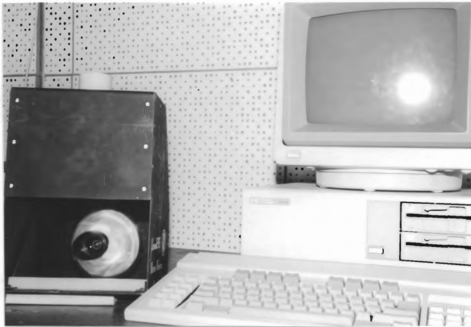
Figure D.1. The "micronEye" camera with computer.
