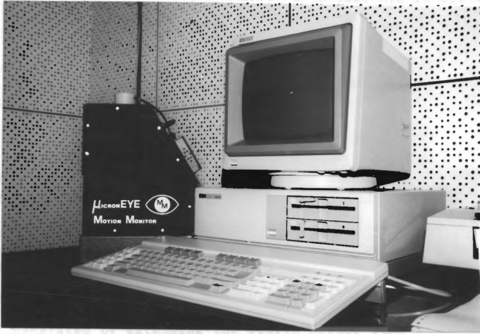
Figure 4.6 The "micronEye" camera with the computer.
