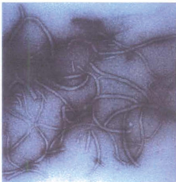
Fig. 3.22 The tubular structure of [\text{Pt}(\text{bipy})\text{H}_2\text{L}]\text{Cl} as seen in a TEM Image (x 73000)
