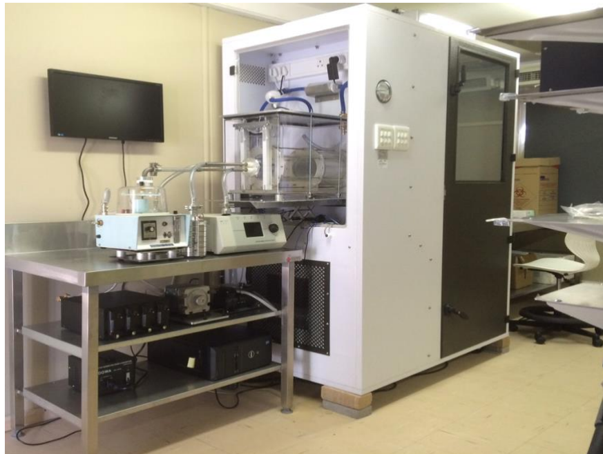
Figure S2.6: The Respiratory Aerosol Sampling Chamber (RASC).
