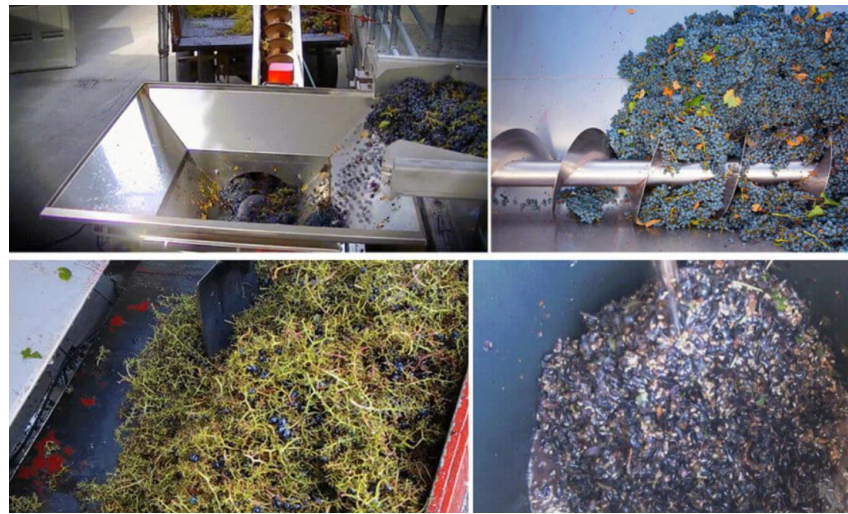
Figure 2-2: Destemming red grapes with the berries sent for processing into wine and the stems taken to landfill sites (Machines, 2019)
