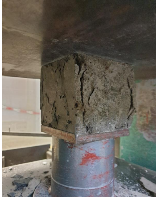
Figure 3-11: Cube failure during loading
