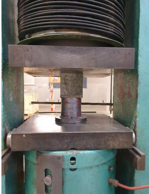
Figure 3-9: Concrete cube undergoing compressive testing
