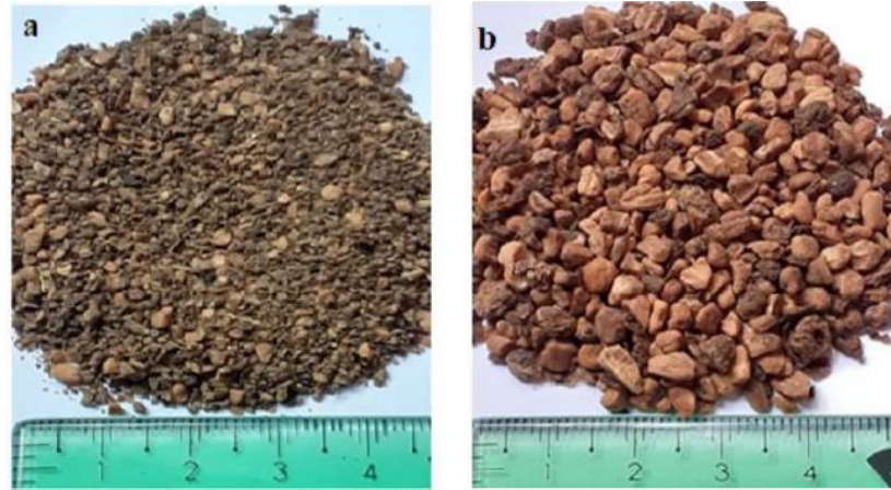
Figure 2-10: Ground olive pomace (a) and ground olive kernels (b) prior to shock-burning (Lila et al. , 2020)
