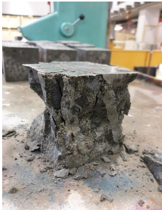
Figure 3-12: Cube failure mode after loading
