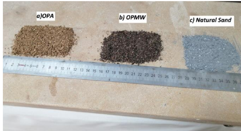
Figure 2-8: Olive pomace aggregates, when dried, have a larger particle size when compared visually to natural sand (Boukhari, 2023)
