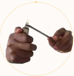
figure 29: flame to steel with no effect to structure. Did not catch fire.
