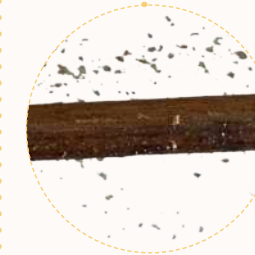
figure 22: timber shavings from friction
