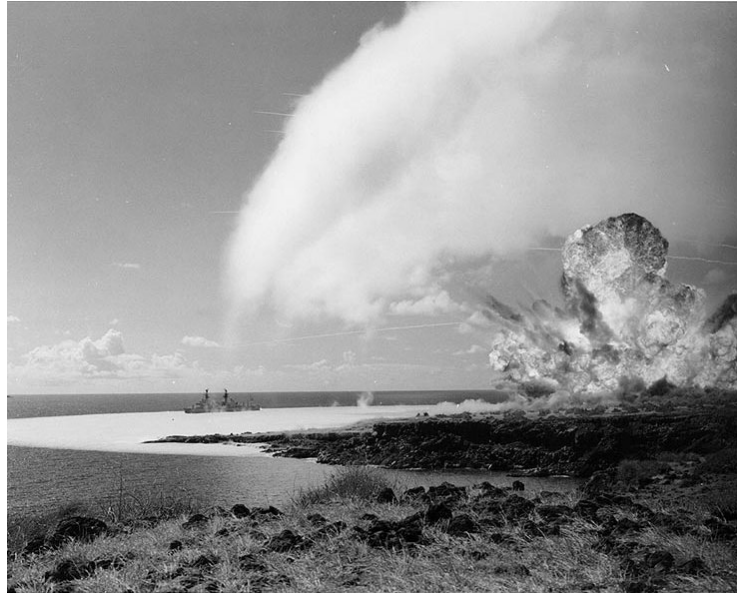
Figure 2.4: A photo of 500 tons of TNT exploding shows the shockwave progress visible on the water and the condensation cloud forming behind it in the air. Operation Sailor Hat, Hawaii, 1965. Courtesy of the US Navy.
