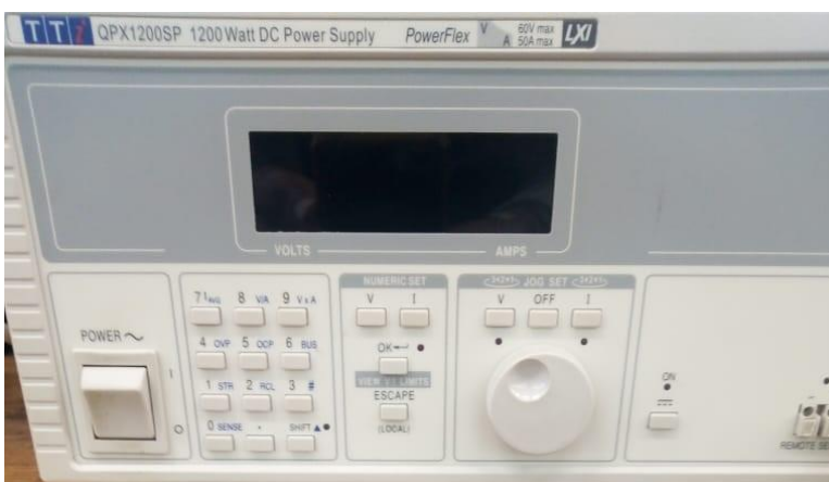
Figure 5.7: dc power supply used to dcGIC injection
