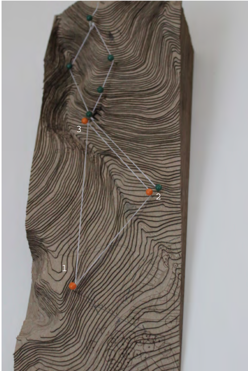
Fig 41. 1:2000 Site model showing the old process in green and the new in orange.(1) Start of the process line. The topography falls from point 1 to 2. (3) The revival of the concrete flumes, water flows down the slope to point 3.
