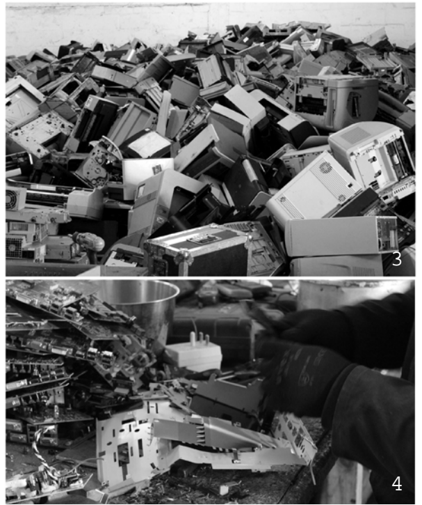
(3) Printers and monitors piled together in stock pile. (4) Manual dismantling of Pc tower. Electronics are transferred from the stock pile to workstations by hand.
