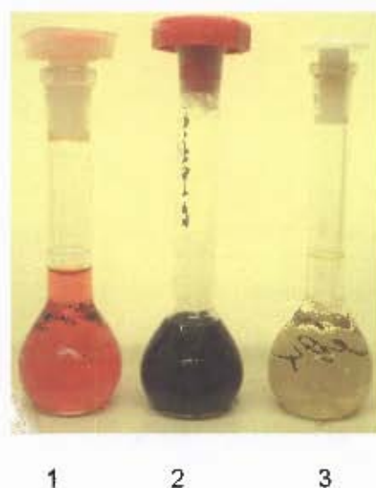
FIGURE 4.6: Solution of receptor (13) during titration with various metal ions in acetonitrile: (1) Solution of S -ferrocenyldithizone (13), (2) Solution of (13) + 2.5 molar equivalent of \text{Hg}^{2+} , (3) Solution of (13) + 2.5 molar equivalent of \text{Cu}^{2+} .
