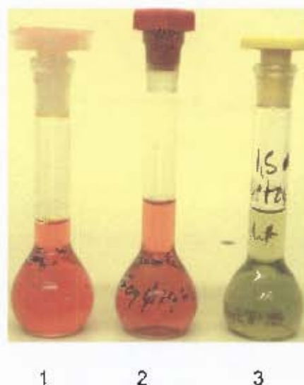
FIGURE 4.14: Solutions of receptor (14) during titration with various metal ions in acetonitrile: (1) Solution of S -ferrocenylmethyldithizone (14), (2) Solution of (14) + 2.5 molar equivalent of \text{Hg}^{2+} , (3) Solution of (14) + 2.5 molar equivalent of \text{Cu}^{2+} .
