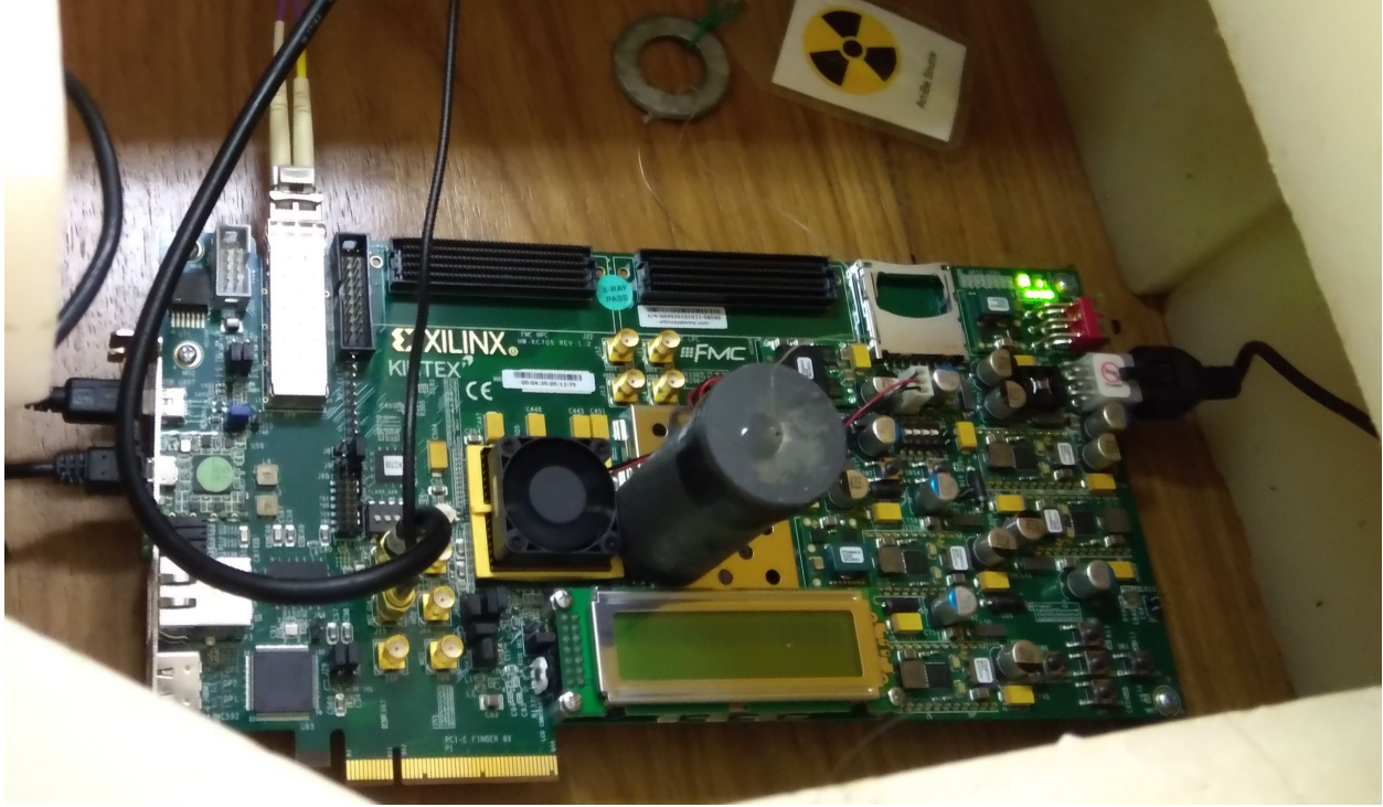
Figure 4.11: Americium-Beryllium cylindrical source placed on a FPGA emulating the EoS lpGBT stages
