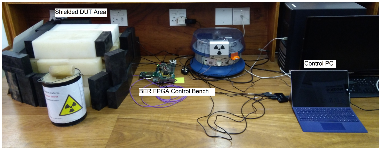
Figure 4.12: Experiment setup with the shielded area which houses the irradiated EoS card or FPGA emulating the EoS shown on the left
