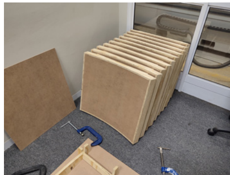
Process Documentation. Cutting, sanding and assembling rectangular panels of Chamber's wall structure.
