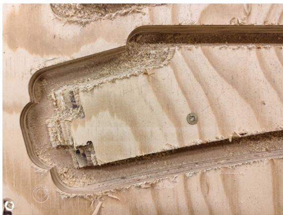
Process Documentation. Results of router malfunction.
