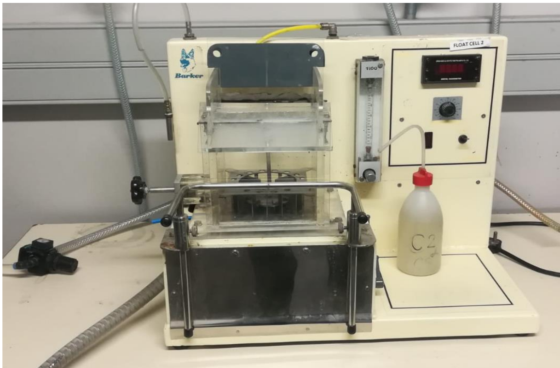
Figure 4.6: 3 L flotation cell used for batch flotation tests.
