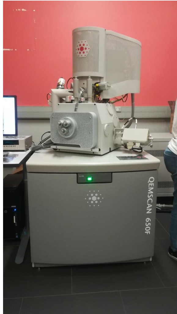
Figure 4.2: QEMSCAN 650F, the mineral analyser that was used in this study.
