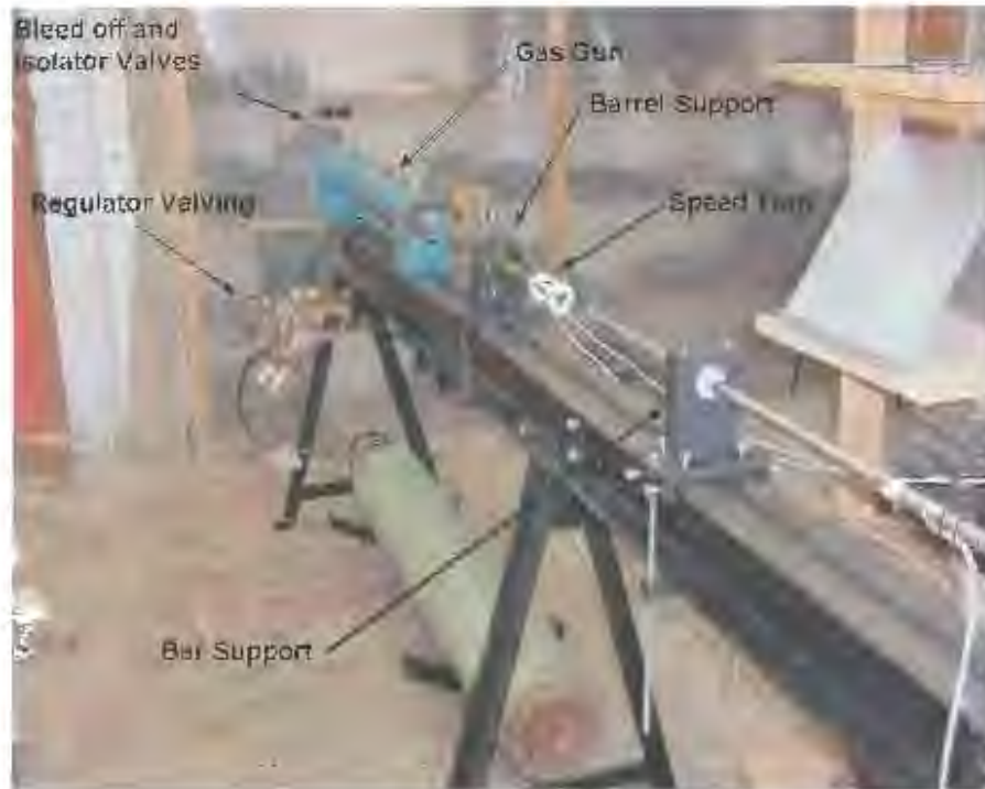
Figure 3-2: Photograph of the compressed gas gun.
