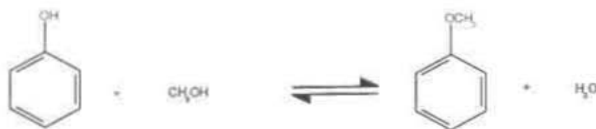
Figure 2.26: Formation of anisole from the methylation of phenol with methanol.
