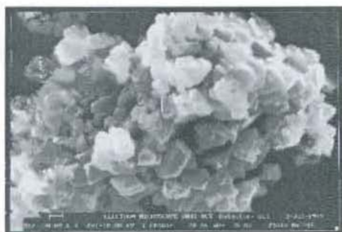
Figure 5.7: Scanning electron micrograph of zeolite H-USY.
