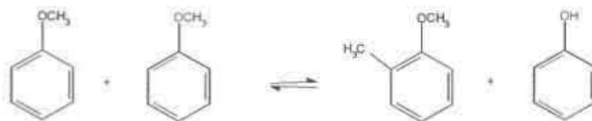
Figure 2.51: Anisole disproportionation to methylanisole and phenol [Marczewski et al. , 1989].
