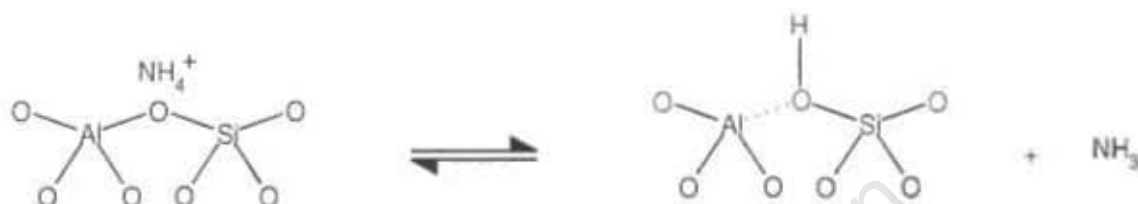
Figure 2.11: Formation of Brønsted acid sites from thermal treatment of the ammonium exchanged zeolite [Nagy et al. , 1998a].
