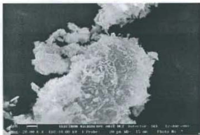
Figure 5.9: Scanning electron micrograph of zeolite H-MCM-22 (DEI).
