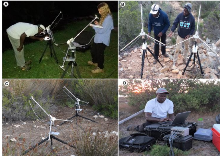
Figure 3.1. The setup of the multiple microphone array system to record echolocation pulses.
