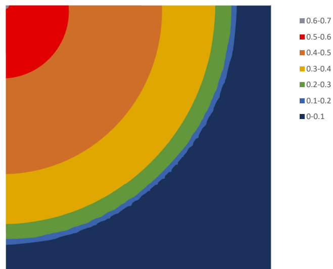
Figure II.14: Saturation profile according to the Richards2D model with base parameters at time t = 8 h and single drip emitter placed on the left.
