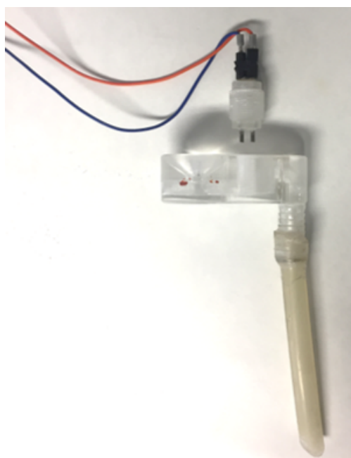
Figure III.4: The photographic picture of the conductivity cell.
