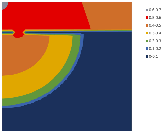
Figure II.17: Richards2D model results with impermeable barrier with a single narrow opening in it.
