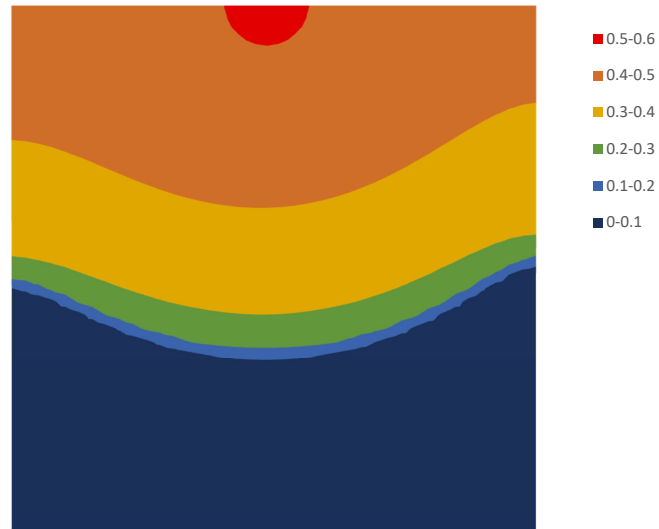
Figure II.13: Saturation profile according to the Richards2D model with base parameters at time t = 8 h.
